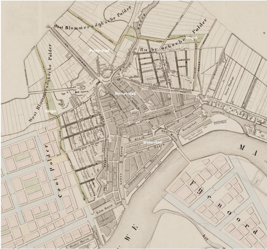
Fig. 4 Detail of the 1858 expansion plan of the city of Rotterdam into the polders, with the new singels to improve the water quality, as part of the water project by city architect Rose. Source Hoogheemraadschap van Schieland en de Krimpenerwaard; released under a Creative Commons Attribution-NonCommercial-NoDerivatives 4.0 International License
