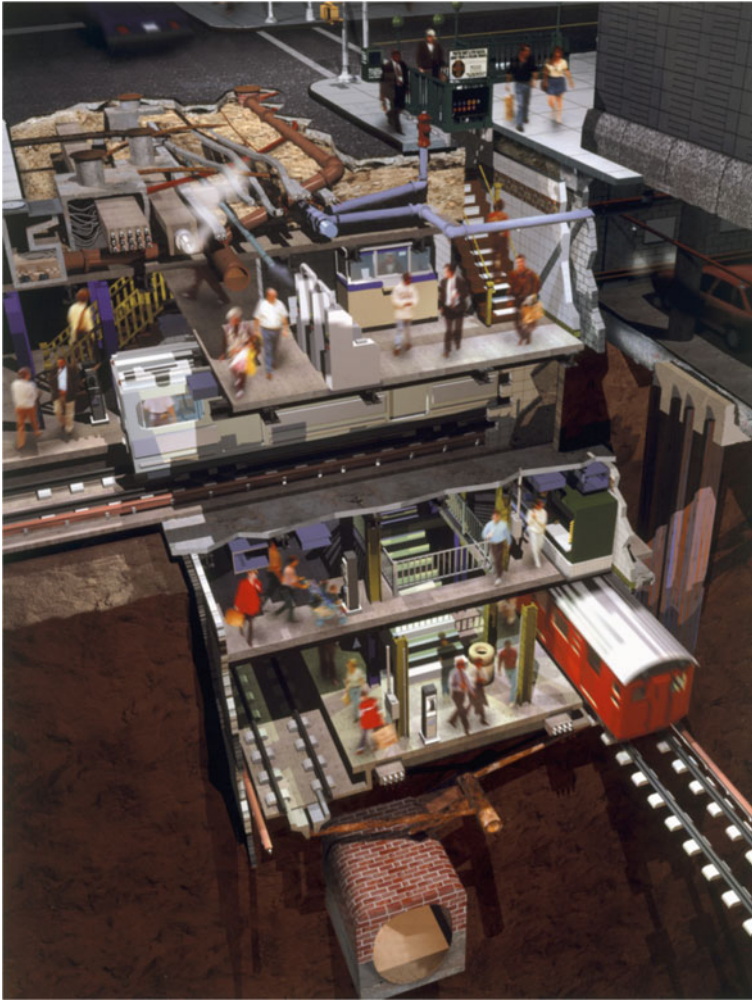
Fig. 1 Axonometric cross section of subgrade infrastructure under a typical Manhattan street. Image courtesy of National Geographic ; all rights reserved
