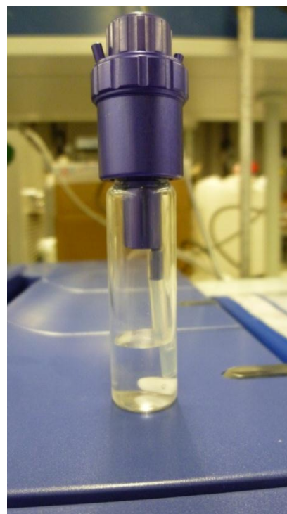
Figure 3.5. Schematic CO 2 purging system and the vial arrangement
