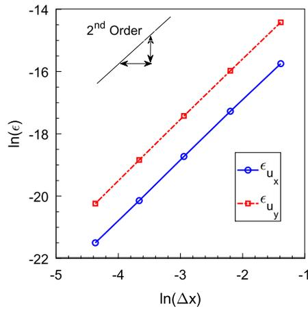
Fig. 3. Second order accuracy of the FVM model.
