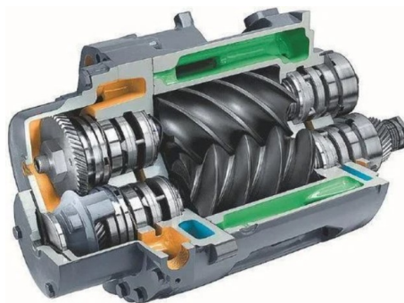
Figure 2.7: Twin-screw compressor with timing gears. Courtesy of Atlas Copco. Figure from D.L.Thurrott (2022).
