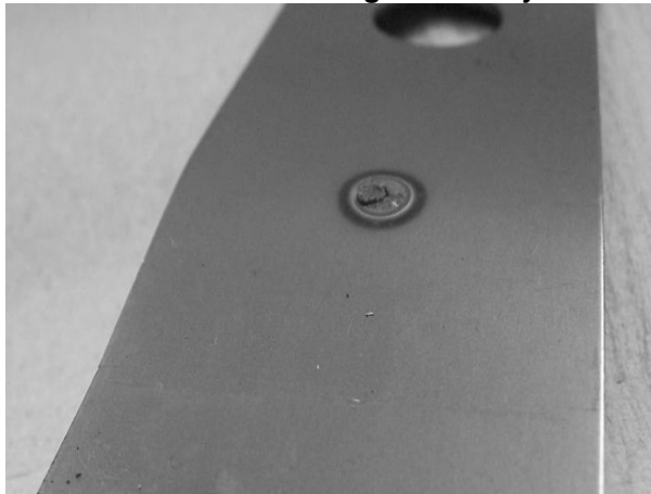
Figure 2.13c: Example of interfacial failure after cross tensile testing of a RSW joint.
