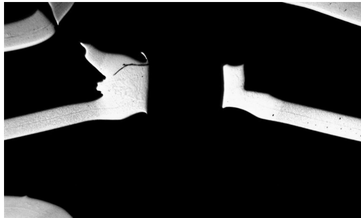
Figure 2.16: RSW joint with centre of weld removed showing failure outside the weld nugget [Den Uijl & Smith, 2006].
