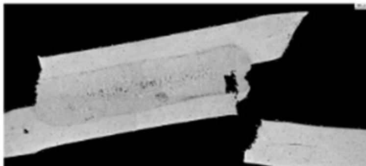
Figure 5.33: weld failure after remelting of the weld nugget edge.
