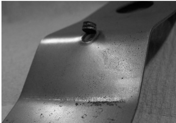
Figure 2.13a: Example of full plug failure after cross tensile testing of a RSW joint.
