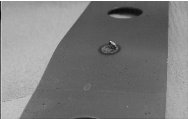
Figure 2.13b: Example of partial plug failure after cross tensile testing of a RSW joint.
