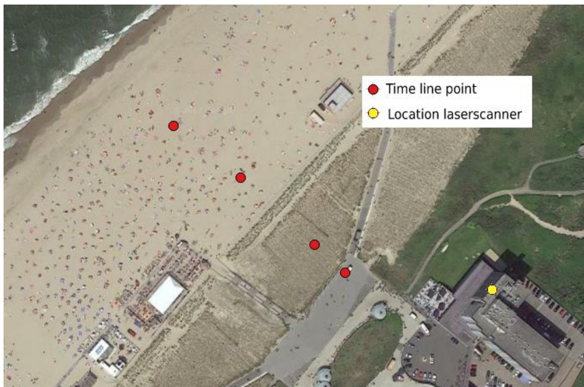
Figure 11. Four different interest points, picked to illustrate differences in time series. From right to left, the yellow dot indicates the location of the laser scanner; the first red point is on asphalt, and assumed to be stable. The second red point is located in the dune vegetation, and is characterized by a high local roughness. The third and fourth point are on the dry part and the intertidal part of the beach respectively.
