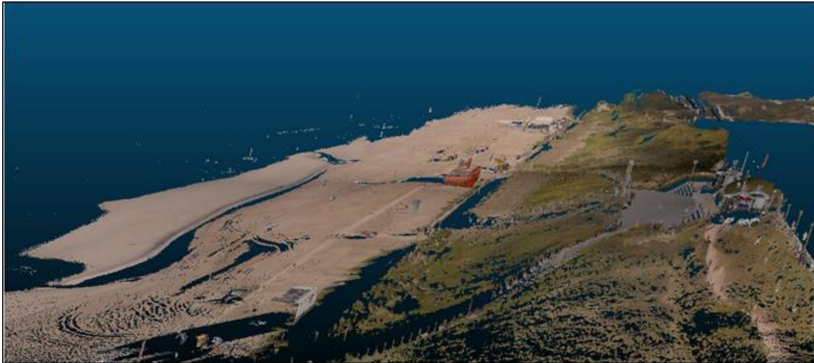
Figure 5. Scan result where each xyz point is colored by RGB information obtained from the built-in true color camera system. The sandy beach on the left is clearly distinguishable from the green dune vegetation on the right.
