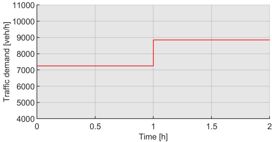
Figure 4.2: Traffic demand flow of all vehicles used as identification demand for the identification of parameters of both case studies
