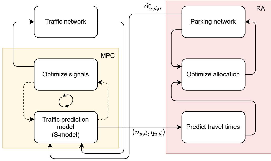
Figure 3.1: Control schemes of MPC and resource allocation where  $\mathbf{x}_{u,d}$  are the traffic states from the traffic prediction model and  $\hat{\alpha}_{u,d,o}$  is the future change in the distribution of the exits
