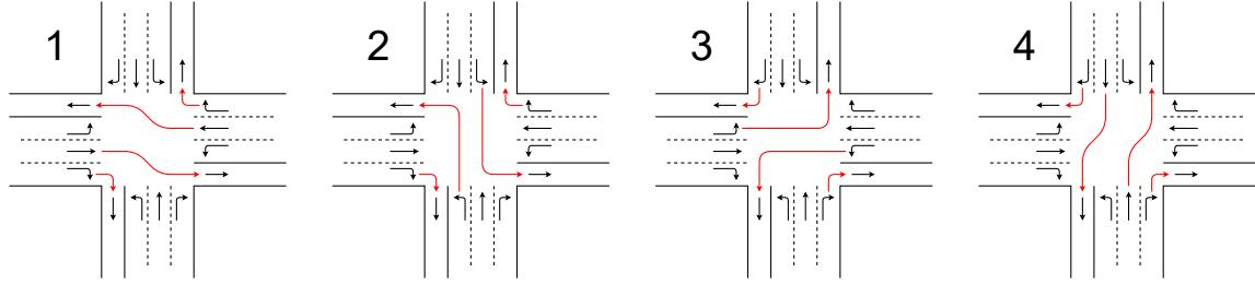
Figure 2.3: Different phases of an intersection, where the red arrows are traffic lights that have right of way
