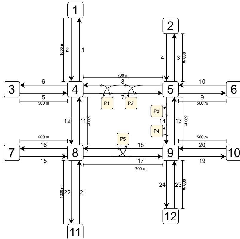
Figure 4.1: Representation of the urban traffic network consistent in the case study
