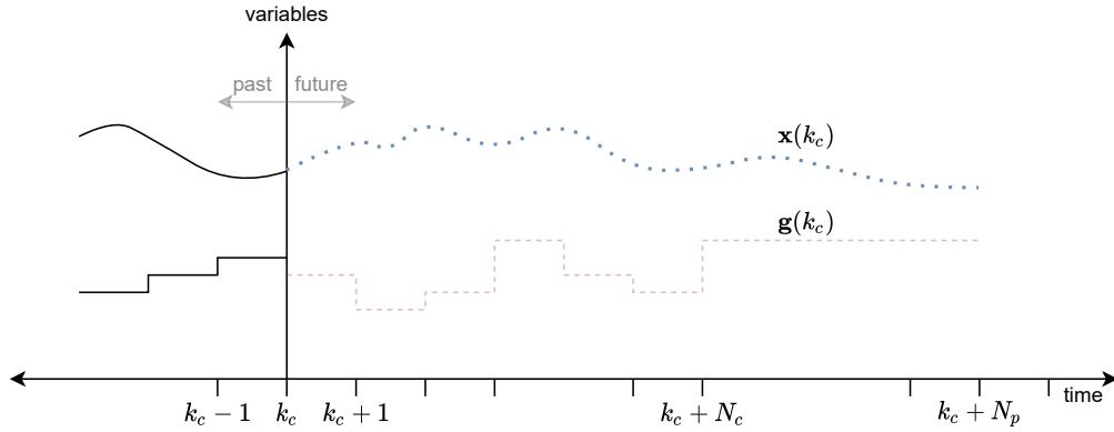
Figure 2.2: Visualisation of the control and prediction horizon  $N_c$  and  $N_p$ , respectively, and the green times  $\mathbf{g}(k_c)$  and state update intervals at every control time step  $k_c$
