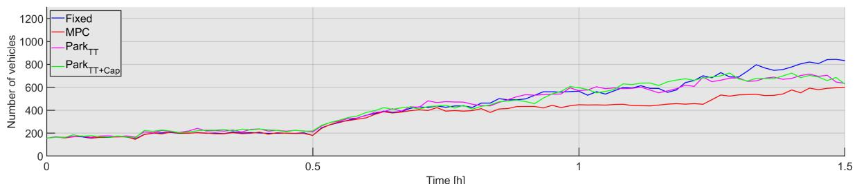
Figure 4.7: The total number of vehicles on the traffic network of all control strategies for the inclining demand scenario of case study A
