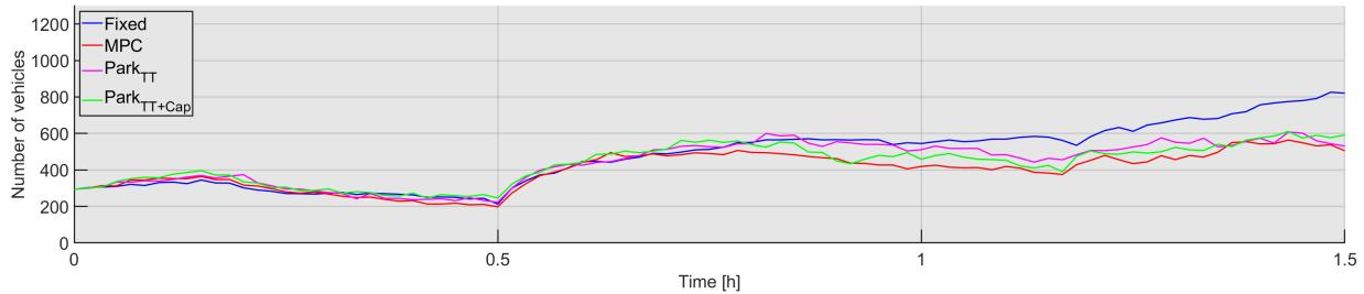
Figure 4.5: The total number of vehicles on the traffic network of all control strategies for the two-peaks demand scenario of case study A
