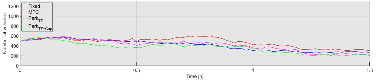
Figure 4.9: The total number of vehicles on the traffic network of all control strategies for the two-peaks demand scenario of case study A
