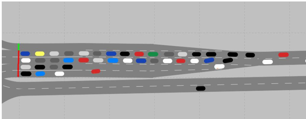
Figure 4.12: An example where the long queue of one exit physically blocks another exit
