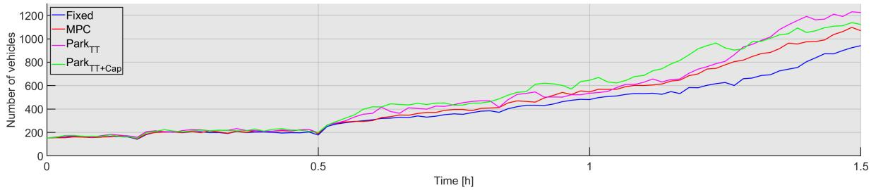
Figure 4.11: The total number of vehicles on the traffic network of all control strategies for the inclining demand scenario of case study B
