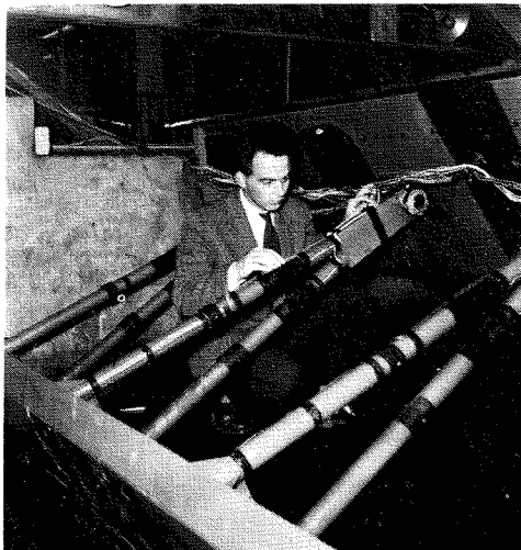
Fig. 13 Elastic similarity model of box girder and one of the tainter gates of the Haringvliet sluices.
