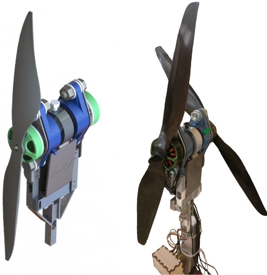
Figure 3-13: Left: perspective render of the T3 CAD design with a single rotor. Right: Constructed T3 experiment in a coaxial testing configuration
