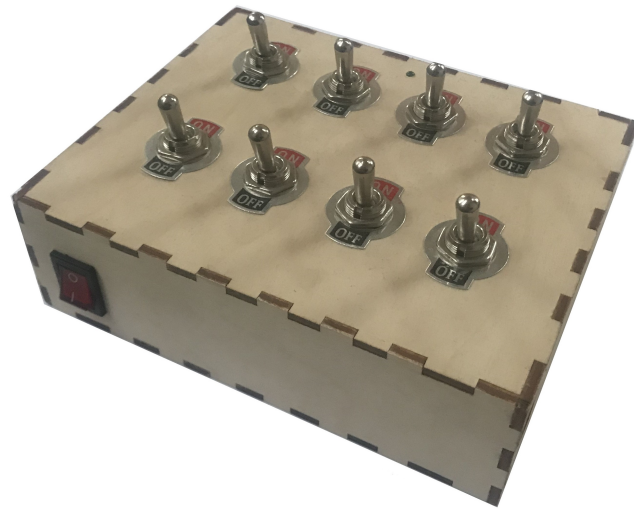
Figure 7-6: Wireless control box comprising 8 toggle switches
