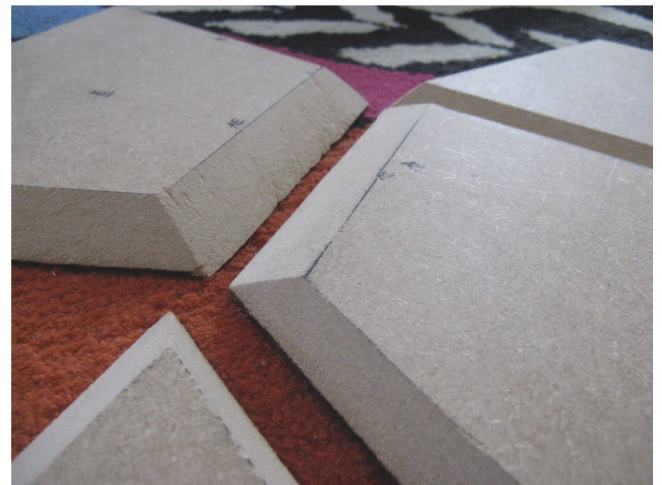
Image 4.12: Close-up of sanded edges of the MDF planes in initial prototype
