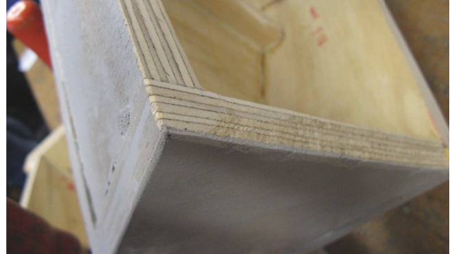
Image 4.14: Detailed view of 18 mm triplex material. Triplex are thinner sheets of wood glued together.
