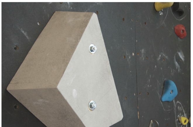
Image 4.16: Finished Block on the climbing wall for user test
