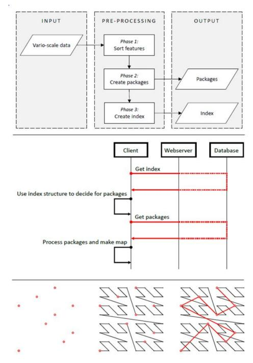
*Figure 3: Methodology of storing vario-scale data and the client-server architecture in three steps (Rovers, 2016).*
