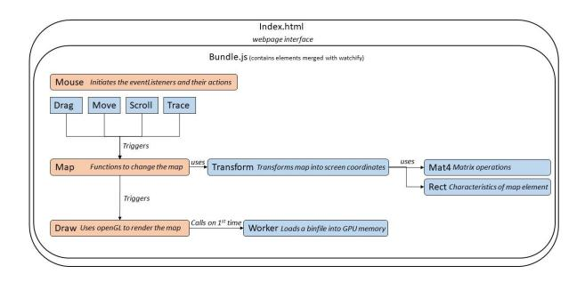
Figure 20: Front-end work principle
