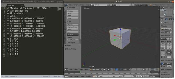
Figure 14. OBJ file format example of a cube
