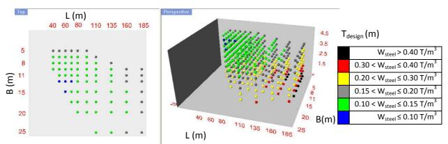
Figure 5-8: Top and 3D-view of steel weight fraction - transversely framed dry bulk vessels
