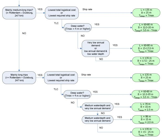
Figure 7-18: Flow chart for the determination of the optimal dimensions of tank ships
