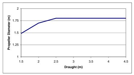
Figure 5-2: Propeller diameter as a function of design draught
