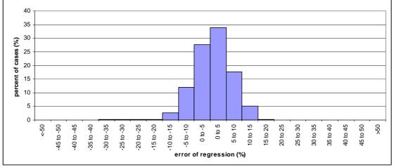
Figure E-2: Steel weight – error distribution for longitudinally framed dry bulk vessels
