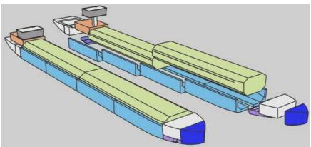
Figure 4-7: Volume subdivision of a typical design
