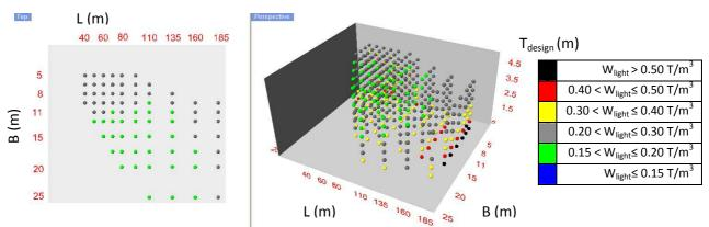
Figure 5-26: Top and 3D views of lightweight fraction as a function of L, B and T<sub>design</sub> - tank vessels
