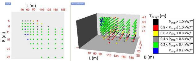
Figure 5-4: Top and 3D-view of installed propulsion power per ton cargo carrying capacity - dry bulk
