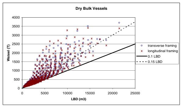
Figure 5-7: Steel weight of dry bulk vessels as a function of LBD
