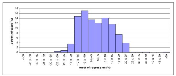
Figure E-13: Piping weight – error distribution for tank vessels
