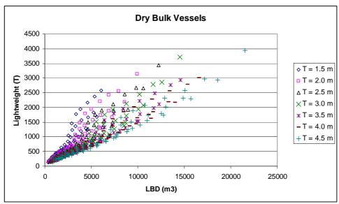
Figure 5-11: Lightweight of dry bulk vessels as a function of LBD
