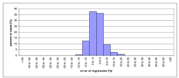
Figure E-3: Piping weight – error distribution for dry bulk vessels
