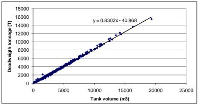
Figure 5-23: Modeled deadweight tonnage vs. tank volume
