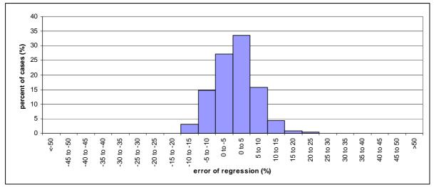
Figure E-1: Steel weight - error distribution for transversely framed dry bulk vessels
