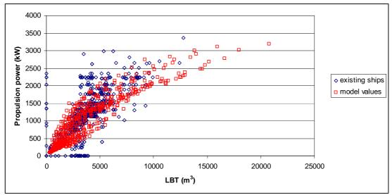
Figure 4-13: Validation of installed power
