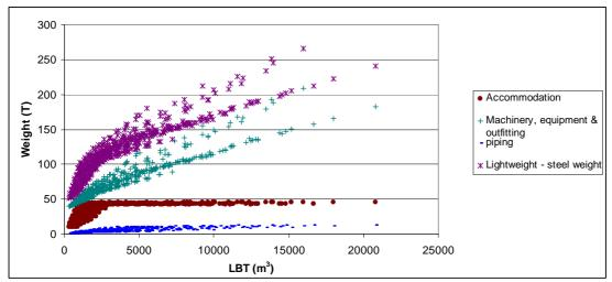
Figure 5-13: Weight of non-structure related lightweight as a function of LBT
