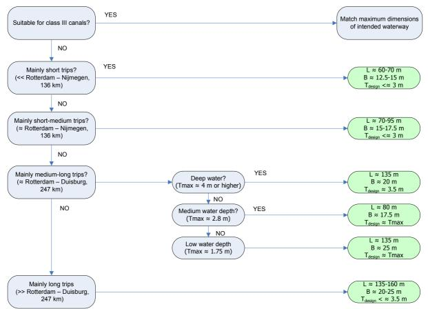
Figure 7-19: Flow chart for the determination of the optimal dimensions of container ships
