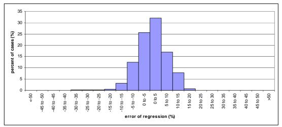
Figure E-9: Steel weight – error distribution for longitudinally framed container vessels
