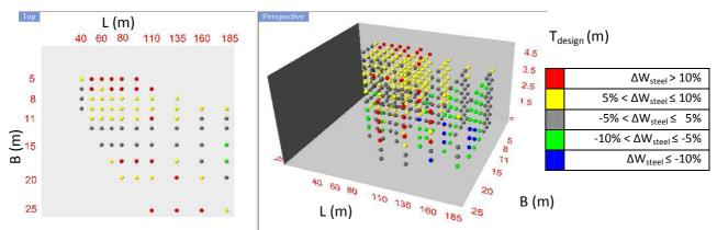
Figure 5-10: Top and 3D-view of difference in steel weight between longitudinally and transversely framed dry bulk vessels
