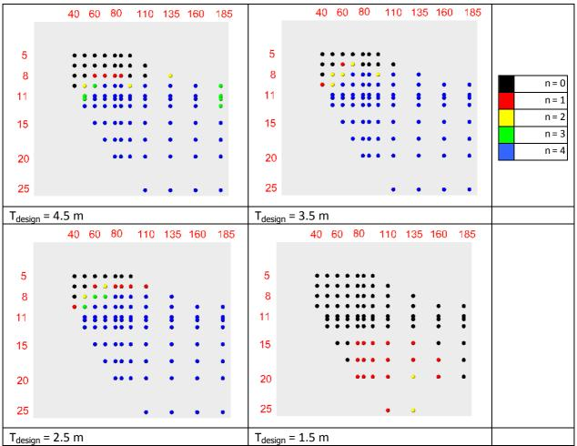
Figure 7-22: Competitiveness of dry vessels with rail – independent of need for end haulage
