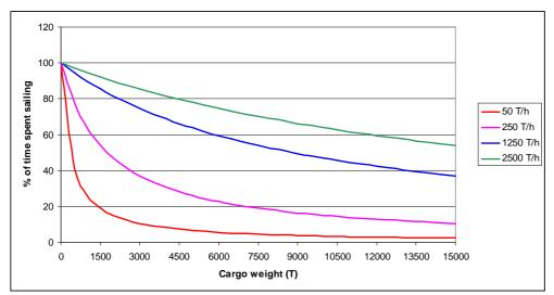
Figure 7-9: Effect of handling speed on percentage of time spent sailing
