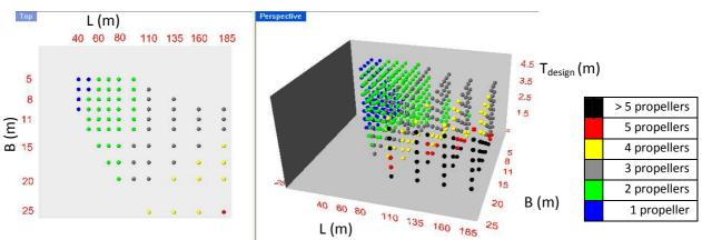
Figure 5-6: Top and 3D-view of the number of propellers as a function of L, B and T
