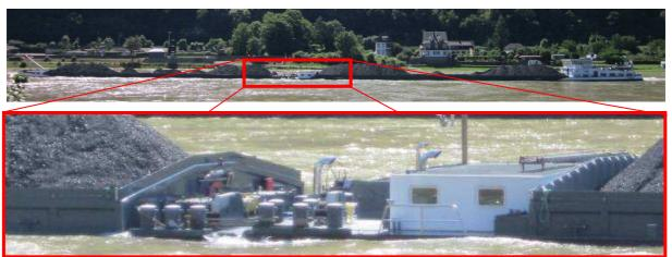
Figure 3-2: Koppelverband Evanti, note the virtual absence of freeboard. Source: own photograph
