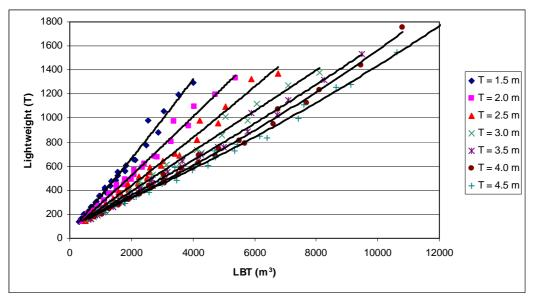
Figure 5-31: Example trend line - lightweight of transversely framed dry bulk vessels
