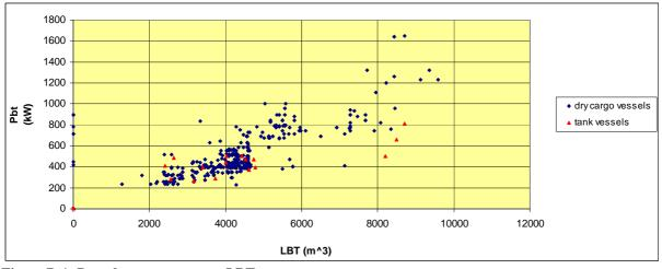
Figure B-1: Bow thruster power vs. LBT
