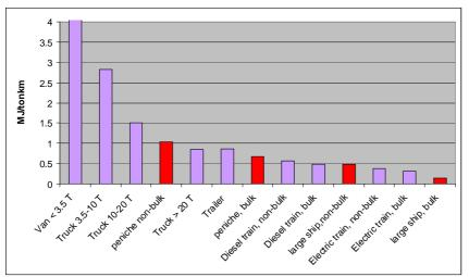
Figure 6-7: Energy consumption of various vehicles and vessels. Source: adapted from CE Delft [2003]
