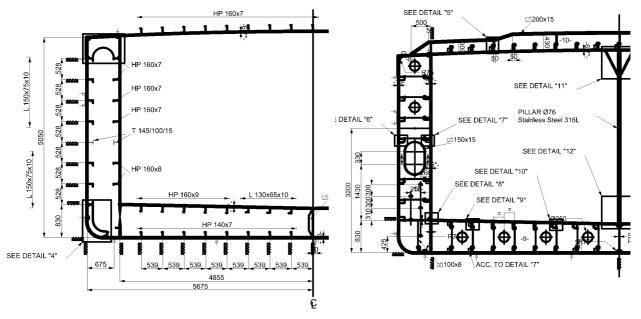
Figure 4-11: Structural drawings of a stainless steel tanker. Drawings courtesy of Mercurius Shipping Group
