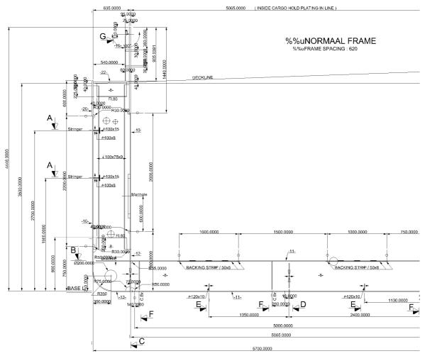
Figure 4-10: Main frame of a dry cargo ship. Drawing courtesy of Mercurius Shipping Group
