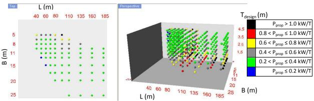
Figure 5-5: Top and 3D-view of installed propulsion power per ton cargo carrying capacity – tank vessels
