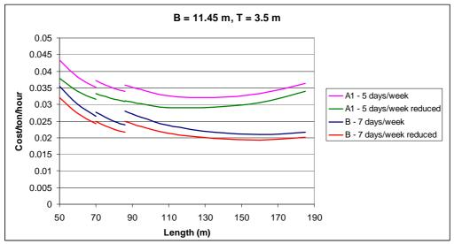
Figure 7-8: Time cost per hour as a function of length
