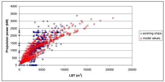
Figure 4-16: Validation of installed power
