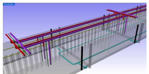
Figure B-3: modeled piping in the midship region of a tank ship
