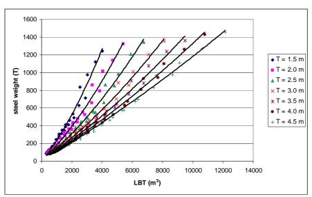
Figure D-1: Steel weight of longitudinally framed dry bulk vessels
