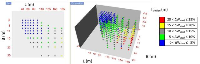
Figure 5-18: Steel weight increase for container vessels compared to dry bulk vessels
