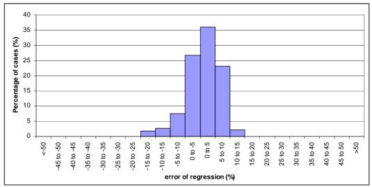
Figure E-10: Yard cost – error distribution for transversely framed container vessels
