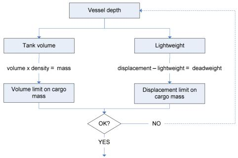
Figure 5-20: Scheme for the determination of vessel depth
