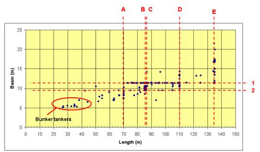
Figure 2-1: Inland vessel main dimensions: L-B Source: own representation of data from [Vereniging 'de Binnenvaart']
