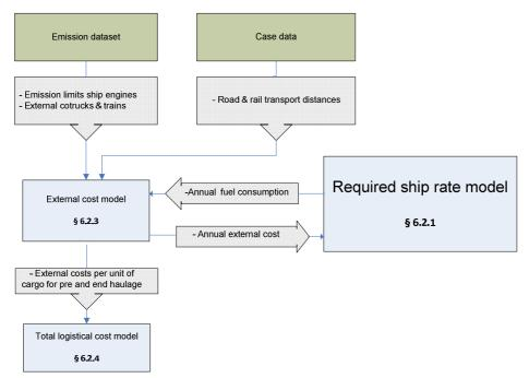
Figure 6-8: Relationship between the external cost model and other sub models
