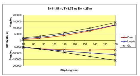
Figure 4-9: Verification of bending moment model
