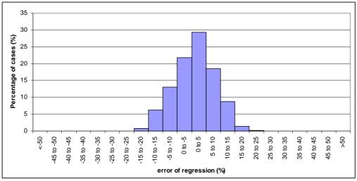
Figure E-11: Yard cost – error distribution for longitudinally framed container vessels
