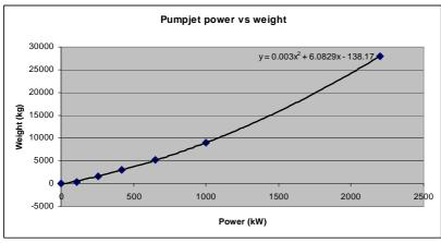
Figure B-2: Bow thruster weight vs. power
