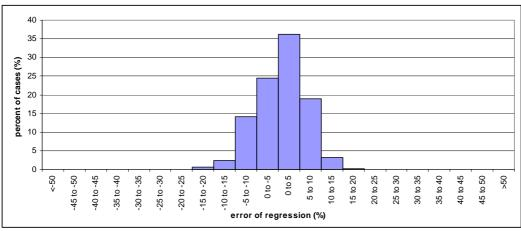
Figure E-8: Steel weight – error distribution for transversely framed container vessels
