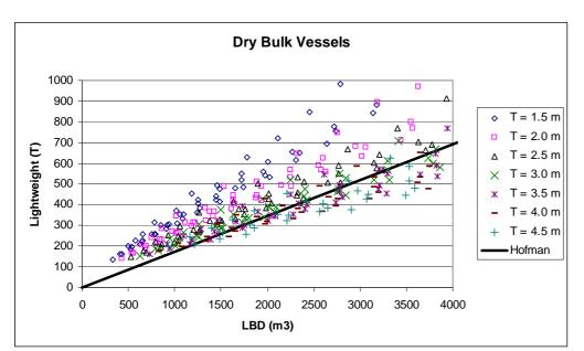
Figure 5-12: Comparison of modeled lightweight with the trend line by Heuser
