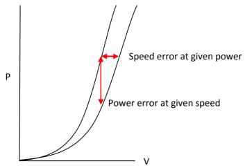
Figure 4-14: Visualization of speed and power errors
