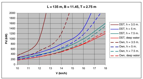
Figure 4-12: Validation of powering calculations
