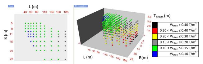
Figure 5-9: Top and 3D-view of steel weight fraction - longitudinally framed dry bulk vessels
