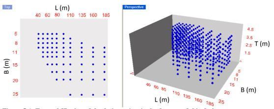
Figure 5-1: Top and 3D-view of the design points in the datasets of ship designs
