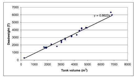
Figure 5-21: Tonnage vs. tank volume for existing ships
