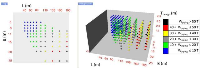
Figure 5-25: Weight of cargo piping for tank vessels
