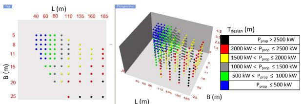
Figure 5-3: Top and 3D-view of installed propulsion power as a function of L, B and T<sub>design</sub>
