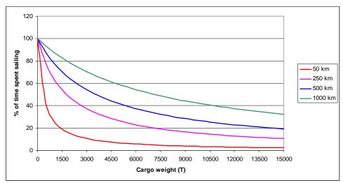
Figure 7-10: Effect of sailing distance on percentage of time spent sailing
