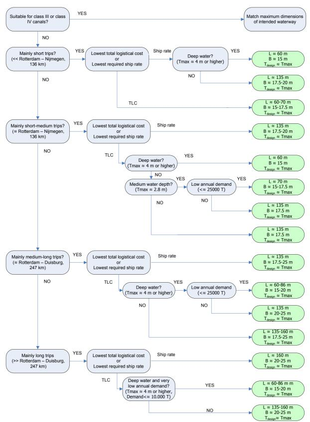
Figure 7-17: Flow chart for the determination of the optimal dimensions of dry bulk vessels
