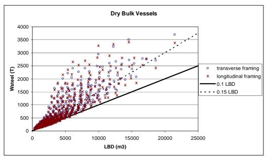
Figure 5-30: Steel weight of dry bulk vessels as a function of LBD
