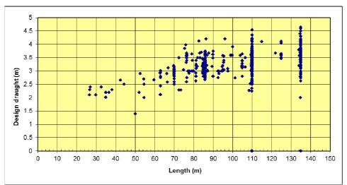
Figure 2-3: Inland vessel main dimensions: L-T<sub>design</sub>. Source: own representation of data from [Vereniging 'de Binnenvaart']
