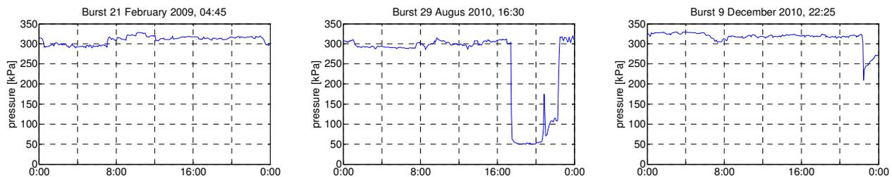
*Figure 7: Pressure near burst locations during burst where the period between occurrence and isolation exceeds 2 hours*
