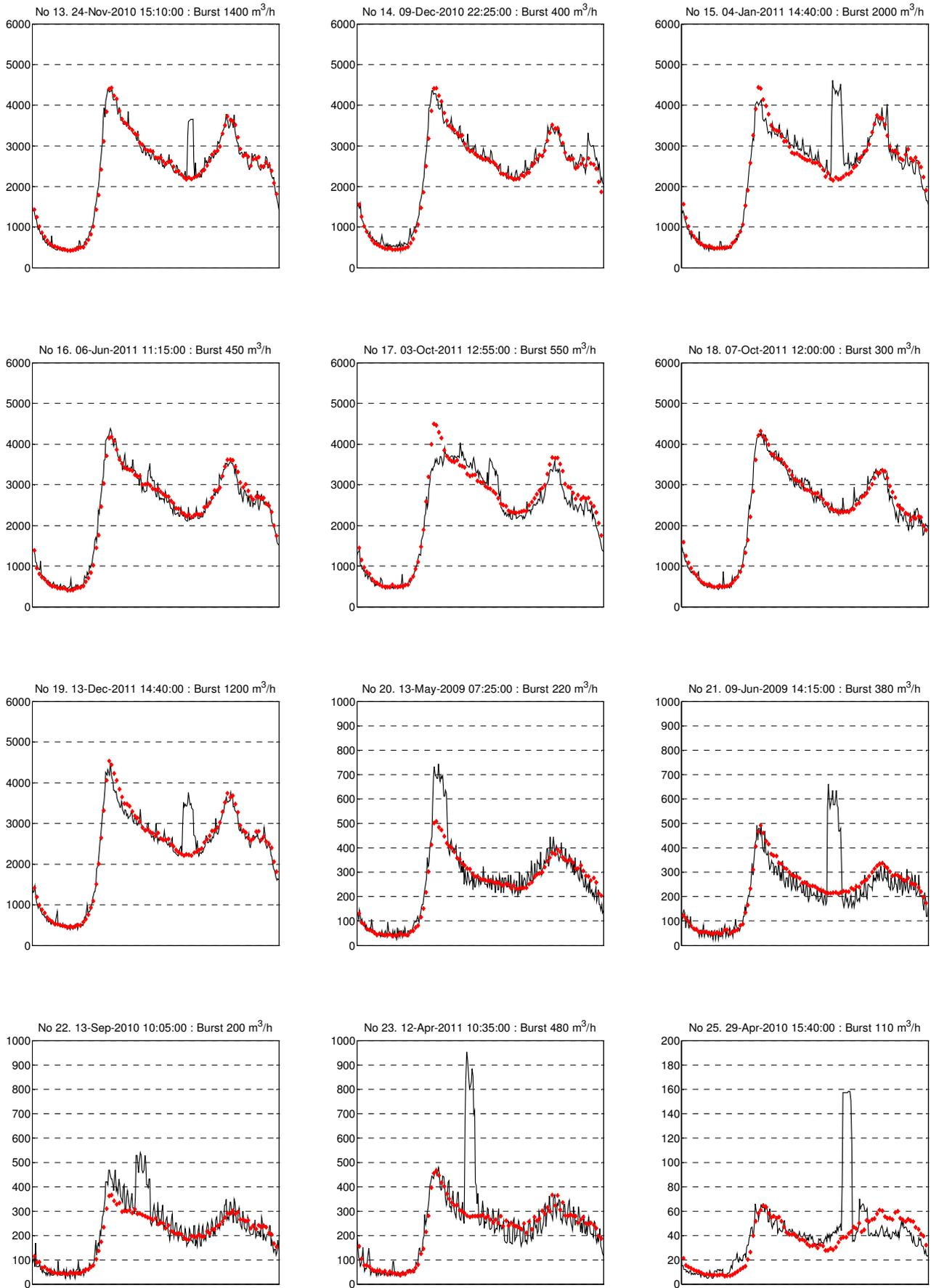
Figure 5: Measured water demand on days with reported pipe burst in 2009-2011 (— = measured flow, ■ = predicted flow). Note that events 20-23 are in Wassenaar and 25 in Noordwijk-HD area.
