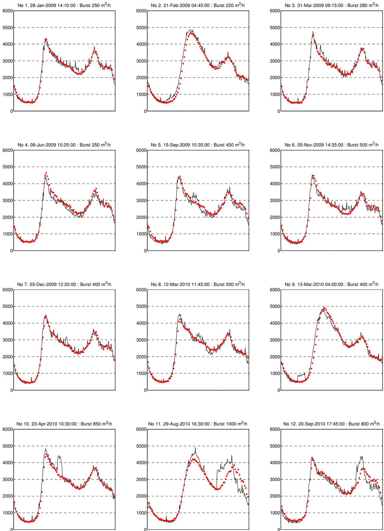
Figure 4: Measured water demand on days with reported pipe burst in 2009-2011 (— = measured flow, ■ = predicted flow).
