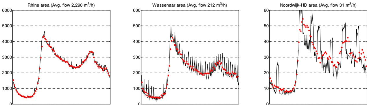
Figure 2: Variability in water demand, in a large area (Rhine area), medium area (Wassenaar area) and small area (Noordwijk-HD area), (— = measured flow, ■ = predicted flow).
