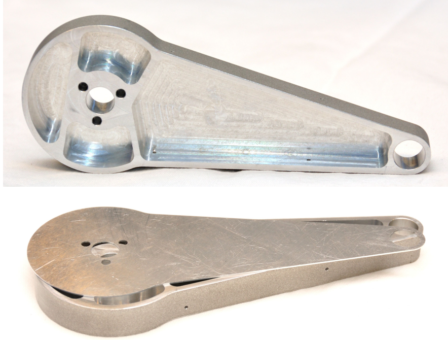
Figure D.5: Lower limb pictures. In the upper picture the inner structure is clearly visible. In the lower picture also the cover plate is shown.
