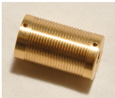
Figure D.13: Picture of the manufactured wire bus. The slots to clamp the wire are still to be made.
