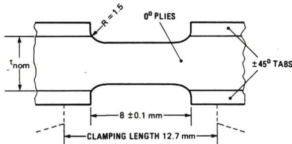
Fig. 2 Detail of DA compression specimen
