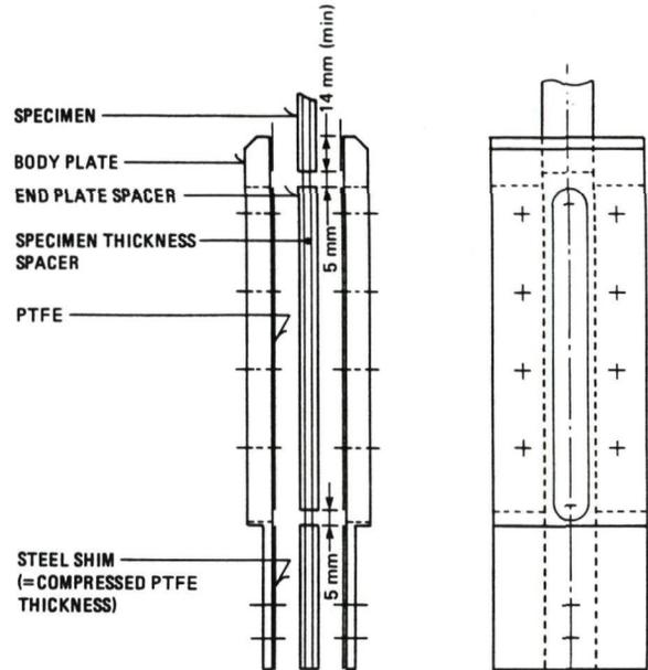
Fig. 3 Anti-buckling guide for multidirectional laminates (CRAG ref. 3)
