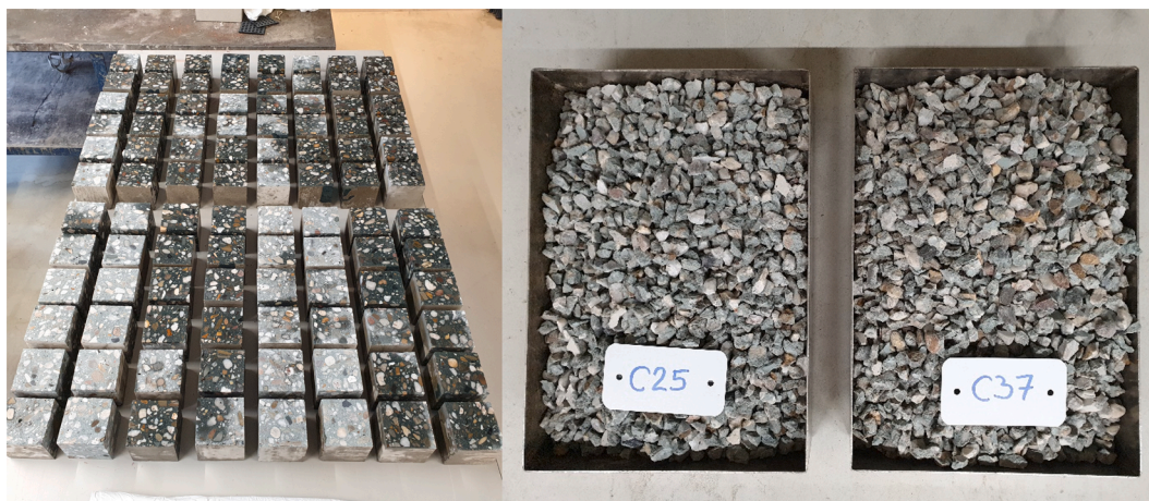
Fig. 2. Specimen preparation: concrete cubes before crushing, RCA after crushing batches C25 and C37.
