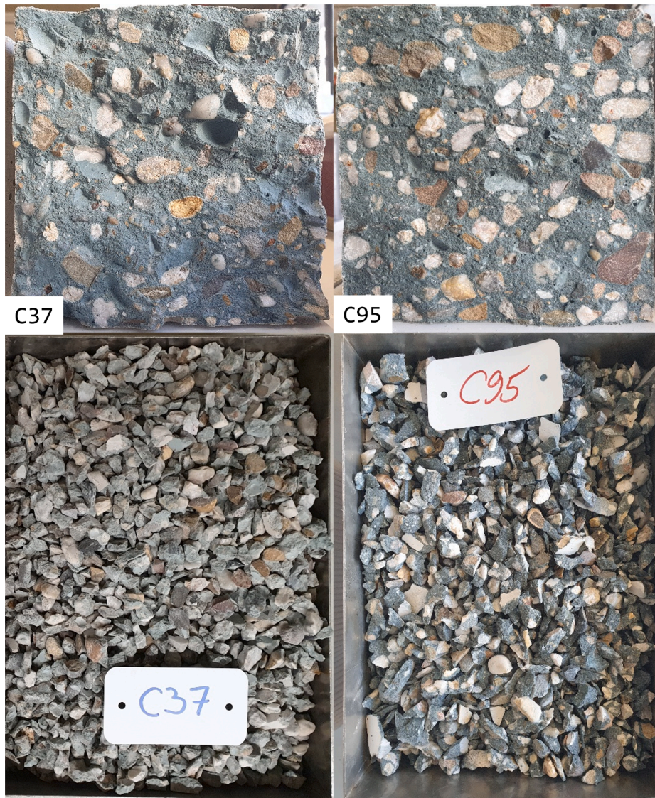
Fig. 9. Fracture in C30/37 and C80/95 specimens after tensile splitting strength test, and shape of RCA sieved for Los Angeles test with a particle size between 10 and 14 mm obtained after dried sieving.
