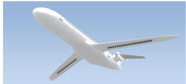
Figure 19: Illustration of the research concept DRAGON showing the integration of DEP on the wing of a Large Passenger Aircraft
