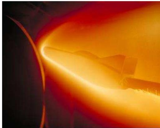
**Figure 1.1:** Aerodynamic heating of M-2 Lifting Body model tested at the Atmospheric Entry Simulator at NASA's Ames Research Center (Image reproduced from NASA gallery)
