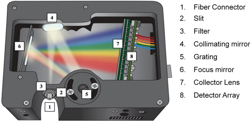
Fig. 3.13: Light enters the spectrometer from a fiber optic cable connected to a probe (1). It is then conditioned by an adjustable slit (2), a filter (3), a collimating mirror (4), and a diffraction grating (5). The grating scatters the different wavelengths onto a focusing mirror (6) that directs the light via a collector lens (7) onto the detector array (8) [16].
