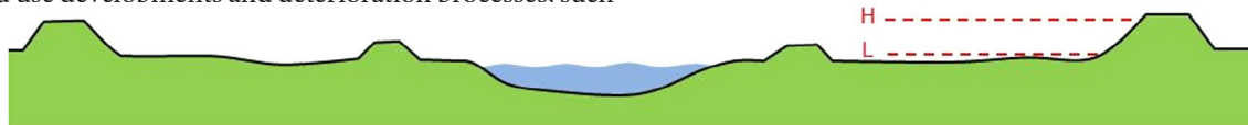
Figure 14. A typical cross-section of the 'present-day' appearance of a river in the Netherlands: a single main channel, low levees ('summer dikes'), flat floodplains and river dikes.
