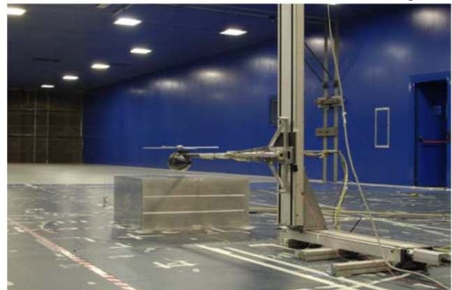
Figure 3. Rotor The rotor-obstacle test setup inside the GVPM wind tunnel (Ref. 22)
