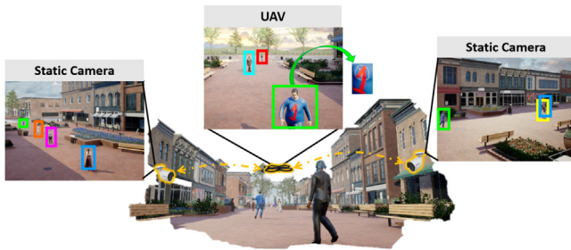
Fig. 1. Overview of our multi-camera collaborative system. The system comprises a camera network that performs a distributed multi-target tracking process. The static cameras monitor the scene and the mobile cameras are guided by a control policy to capture close-up images of viewpoints likely to strengthen the classification of certain attributes.
