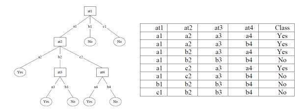
**Figure 3-1:** Decision tree for the training set with classes Yes and No. The instance [at1=a1, at2=b2, at3=a3, at4=a4] sorts to the nodes at1, at2 and at3, classifying the instance as positive represented by the value "Yes" [6].
