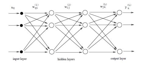
**Figure 3-2:** Feed-forward Artificial Neural Network, allows signals only to travel forward from input to output [32].
