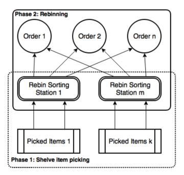
**Figure 1-1:** Vanderlande order picking process scheme. In phase 1 items are picked from shelves, placed in a bin and transported to a rebin sorting station. In phase two a manual worker scans each item from a bin and places it in its responding order destination.
