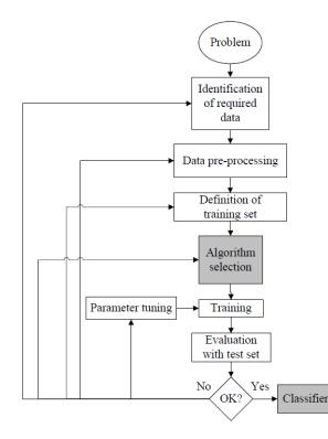
Figure 2-1: Supervised machine learning pipeline that is used to create a successful classifier [6].
