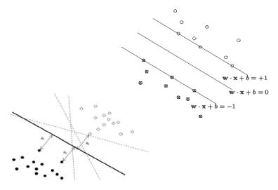
Figure 3-3: Creating the optimal separating hyperplane with the use of support vectors [9].
