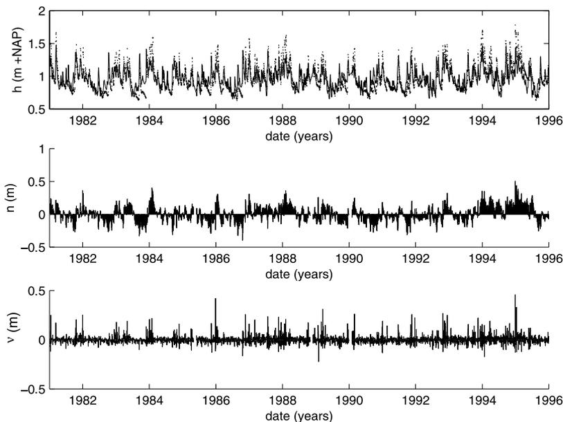
**Figure 5.** Time plot of the available groundwater level observations (dots) from piezometer 32cl0034 relative to the national reference level (h+NAP), the predictions of the transfer model (solid line), the model residuals ( $n$ ), and the innovation series ( $v$ ).
