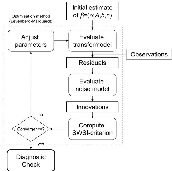
**Figure 4.** Procedure for applying the noise model in combination with a deterministic model.
