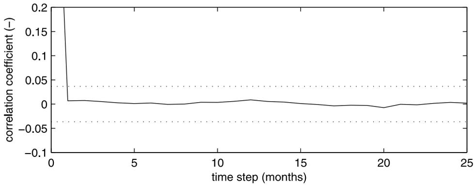
**Figure 6.** Autocorrelation function of the innovations of the OUB model. The dotted lines denote the 95% confidence interval. The autocorrelation function indicates that the white noise assumption holds.
