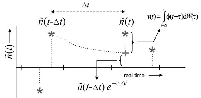
**Figure 3.** Schematic representation of the functioning of an exponential noise model in continuous time. The star denotes a residual, whereas the plus denotes a predicted residual. The model directly predicts the value of the residual series for the next observation available.
