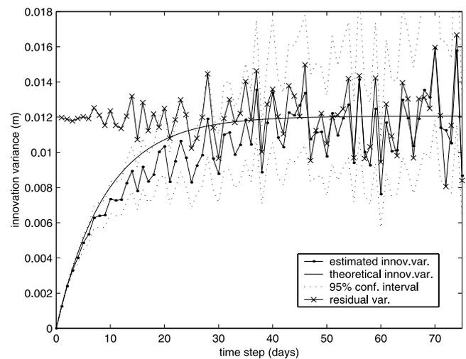
**Figure 9.** Plot of the estimated and theoretical IVF as a function of the time step and of the estimated residual variance. In general, the estimated innovation variances do not differ significantly from the theoretical IVF, although the agreement is better for smaller time steps.
