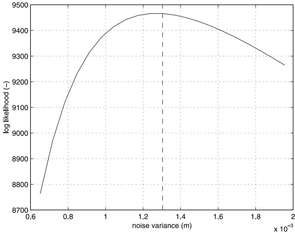
**Figure 8.** Plot of the log likelihood function of the innovations as a function of the parameter  $\sigma_a^2$ . The dashed line denotes the value of  $\sigma_a^2(\beta)$  obtained with the SSWI criterion. The minimum of the log likelihood function proves to coincide well with the value obtained from the SSWI criterion.
