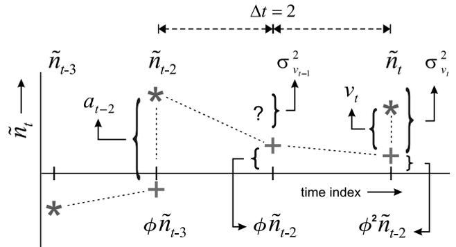
**Figure 2.** Schematic representation of the functioning of an AR(1) model combined with a “degenerate” Kalman filter. The star denotes a residual, whereas the cross denotes a predicted residual. The model predicts missing values of the residual series at every time step, along with the prediction error variance.
