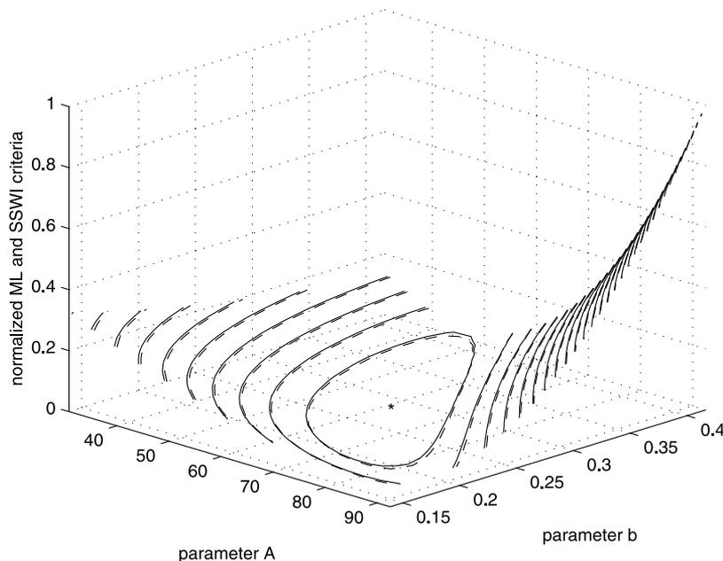
**Figure 7.** Contour plot of the normalized log likelihood function of the innovations (dashed lines) and the SWSI criterion (solid lines) as a function of the parameters  $A$  and  $b$  (all other things kept constant). The star denotes the estimated values. It can be seen that both functions are almost identical.
