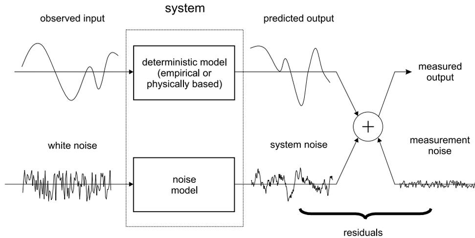
**Figure 1.** Schematic representation of a combined deterministic-stochastic model of a system under the influence of system noise, measurement noise, and a deterministic signal.
