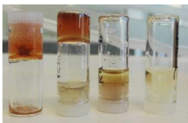
Figure S6.23. Critical gelation concentration tests with gelator 1b . Concentrations of 1b from left to right: 20 mM, 30 mM, 10 mM, 1 mM. The images show that the CGC of 1b is between 10 and 20 mM. The precipitate in the first vial is caused by mechanical disturbances. 0.18 eq. Rh-catalyst and 90 eq. sodium formate are added compared to [ 1a ].
