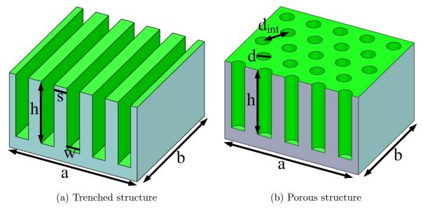
Figure 3.10: Schematics of surfaces with high AR structures: (a) trenched, (b) porous. The effective area is highlighted in green.
