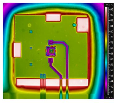
Figure 5.11: Thermal image of WLP on thermal insulator (cardboard) after 20 min.
