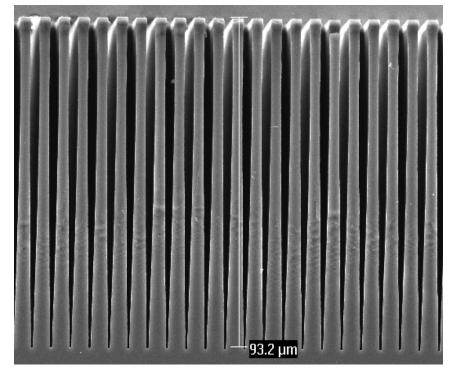
Figure 3.14: Effects of ARDE during high AR trench etching.
