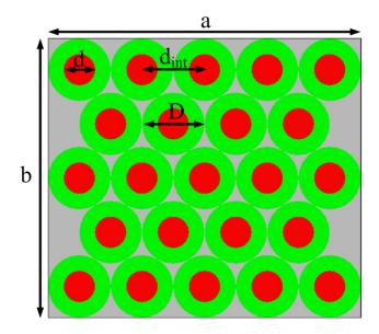
Figure 3.11: Hexagon pore layout. Red circles are the pores, green – tangent circles with  $D = d_{int}$ .
