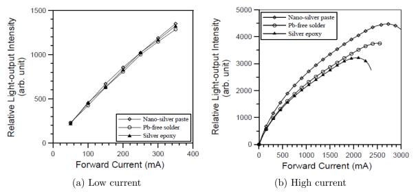
Figure 1.3: Relative light intensity of LEDs attached using three different materials at (a) low and (b) high supplied current values [34].
