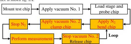
was used to adjust the  $N_2$  flow necessary to bend the chip. A diagram of the measurement sequence is shown fig. 5.4.
