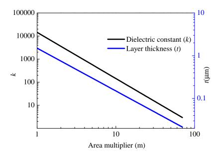
Figure 3.13: Dielectric constant and layer thickness (right axis) required to integrate  $68 \,\mu\text{F}$  as functions of area multiplier.
