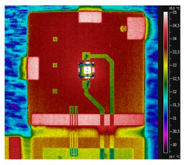
Figure 5.10: Thermal image of WLP on metal chuck after 20 min.
