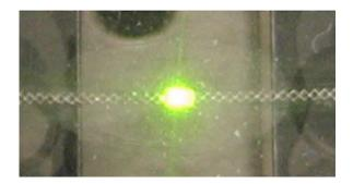
Figure 2.5: PDMS encapsulated LED with EGaIn diamond-shaped interconnects [57].
