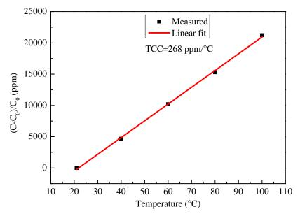
Figure 5.8: Temperature dependency of normalized capacitance. CC=0.99.
