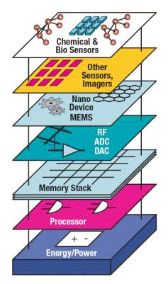
Figure 1.2: Functionality stacking for 3D integarion [8].
