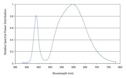
Figure 5.12: Relative SPD of while LED with CCT=3000 K [104] at 25 °C.
