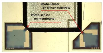
Figure 1.8: Top view of MSM sensors on Poly-Si membrane and Si surface.
