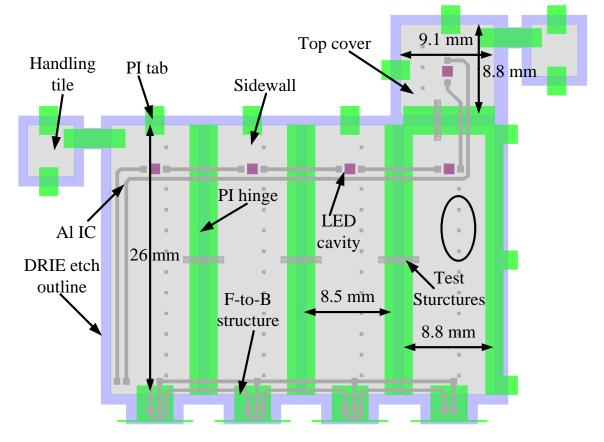
Figure 2.8: Front-side layout of proposed WLP design.
