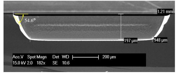
(b) Cross-section of DRIE etched cavity
