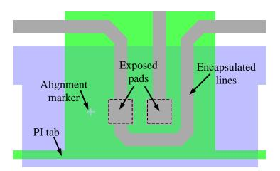
Figure 2.11: Polyimide based front-to-back interconnect structure.
