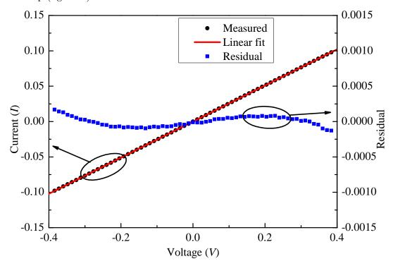
Figure 4.13: Continuity validation of the flexible front-to-back interconnection structure by I - V sweep. Linear fitting with correlation coefficient=1 was obtained.
