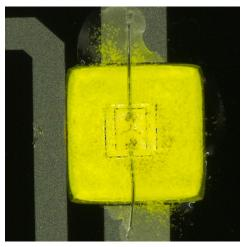
(a) LED cavity filled with phosphor
