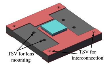
Figure 1.5: Wafer level package with TSVs for electrical connections and micro-lens attachment.
