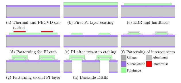
Figure 2.15: Flexible interconnect fabrication process.
