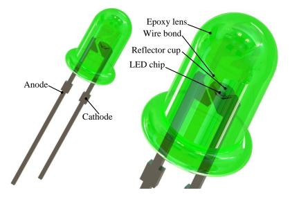
Figure B.2: Low power lead frame through-hole LED.
