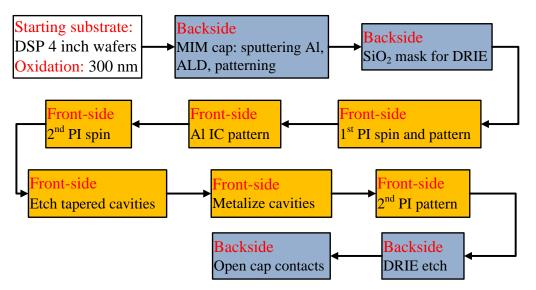
Figure 4.3: Schematic diagram of the 3D WLP fabrication flow.
