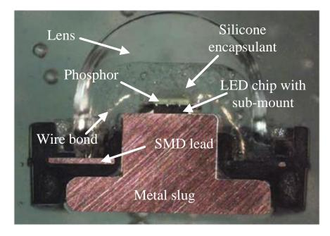
Figure B.3: Cross-section of HB LED package from Lumileds [22].
