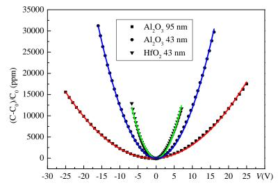
Figure 5.6: C-V of thermal and PEALD Al<sub>2</sub>O<sub>3</sub> and HfO<sub>2</sub> MIM capacitors.
