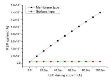
Figure 1.9: Photo-current generated by MSM sensors fabricated on poly-Si membrane and Si surface with increasing LED driving current.
