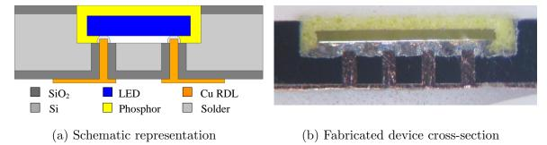
Figure 1.4: Flip-chip WLP with Cu pillars and RDL [35].
