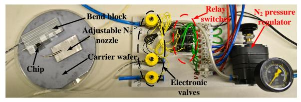
Figure 5.3: Bending test sequence.
