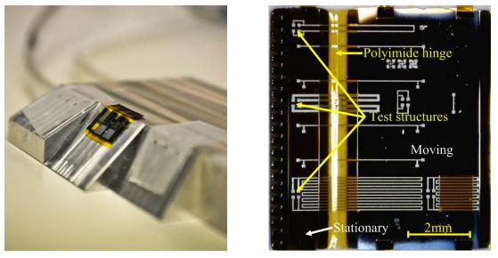
(a) Test chip on bending block.
