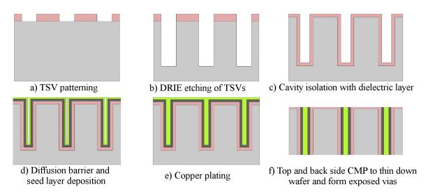
Figure A.1: TSV fabrication process flow.
