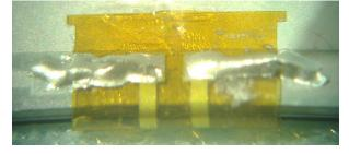
Figure 4.12: Glued and connected flexible front-to-back structure.
