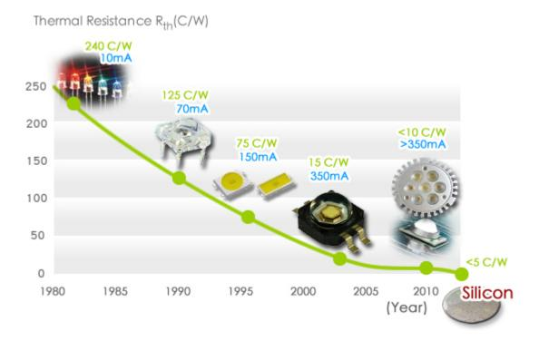
Figure B.1: Development of LED packages in terms of reduction in thermal resistance. (Source: http://www.viseratech.com)
