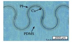
Figure 2.4: PI-enhanced stretchable interconnects [55]
