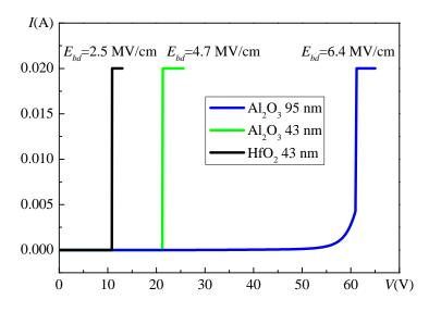
Figure 5.7: Dielectric breakdown of thermal and PE ALD Al<sub>2</sub>O<sub>3</sub> and HfO<sub>2</sub> MIM capacitors.
