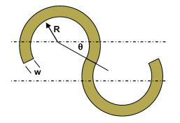
Figure 2.3: Horseshoe meander shape: R – inner diameter, W – line width,  $\theta$  – joining angle [48]
