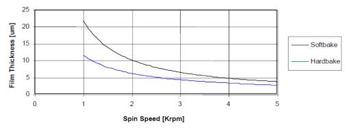
Figure 2.16: PI 115A spin curve [63].
