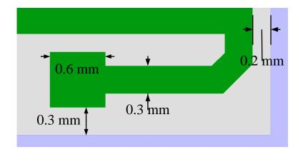
Figure 3.6: Dimensions and spacings on the edge of capacitor plate.
