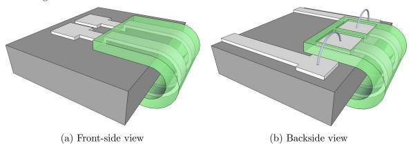
Figure 2.12: Schematic representation of front-to-back interconnection
