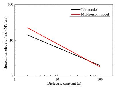
Figure 3.9: Models predicting the breakdown strength of dielectric materials as a function of k [88, 89] on a log-log scale.
