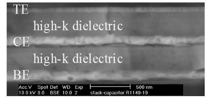
Figure 3.3: A parallel capacitor stack, with CE being the shared plate. MIMIM structure. and breakdown voltage of 90 V. BaSrTiO<sub>3</sub> films with k=420 have been employed for tunable
