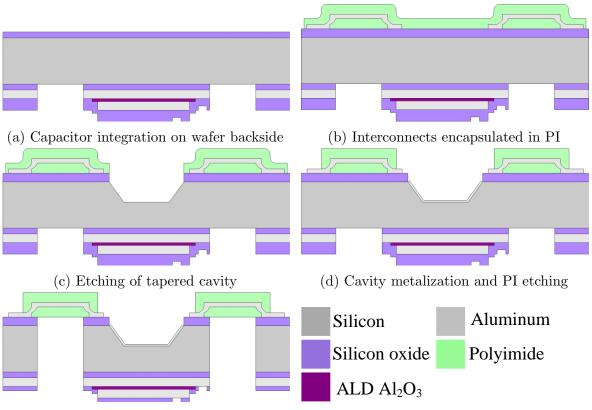
(e) Cavity metalization and PI etching
