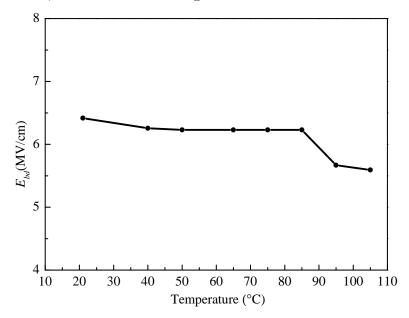
Figure 5.9: Temperature dependency of dielectric breakdown.
