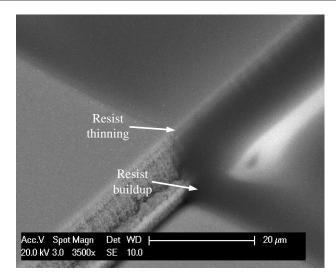
Figure 2.21: Step coverage of 3 µm photoresist indicating the non-uniform layer thickness along the PI slope.
