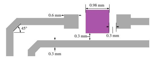
Figure 2.9: Dimensions of package interconnects and LED cavities.
