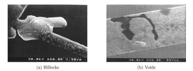
Figure 2.6: Interconnect defects caused by electromigration [58]
