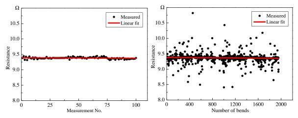
(a) Resistance measurements before bending. (b) Bending test results after 2000 cycles of 90 degree bends.
