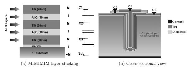
Figure 3.4: 3D MIM trench capacitor: (a) the schematic of the stacked structure. Highly doped substrate wafer is used as bottom electrode. (b) Cross-section schematic.
