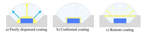
Figure C.1: Phosphor dispense methods: a) freely dispensed phosphor, b) conformal coating, c) remote coating. Color shifts for each method are also show.
