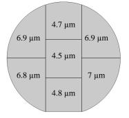
Figure 2.20: Non-uniformity of isotropic etching with barrel etcher.
