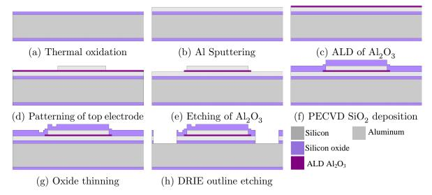
Figure 3.7: MIM capacitor fabrication process.
