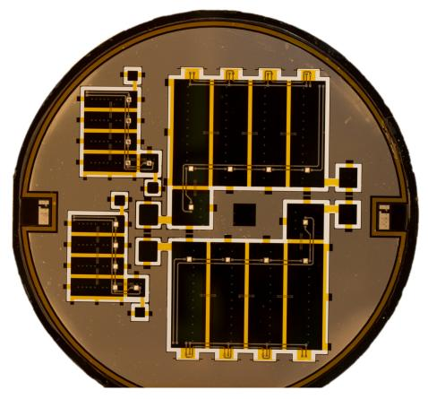
Figure 4.4: Fully fabricated packages on Si wafer.
