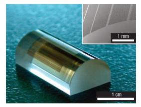
Figure 2.1: Thin silicon structures on spherical surface, applied by transfer printing [48]
