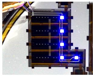
Figure 4.5: Current supplied to wire bonded LEDs.
