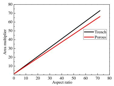
Figure 3.12: Comparison of area gain from increasing the structure AR for porous and trench designs.
