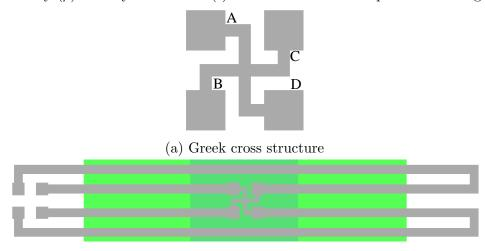
(b) Greek cross structure encapsulated in PI hinge
