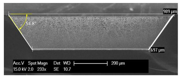
(a) Cross-section of KOH etched cavity
