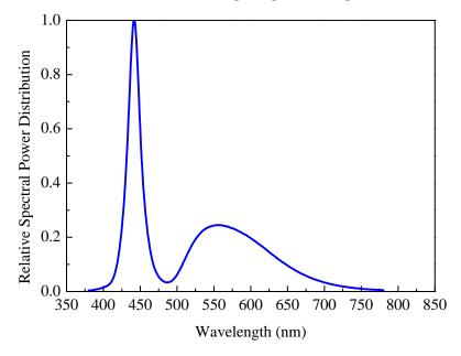
Figure 5.13: Relative SPD of fabricated WLP at 25 °C after color conversion.
