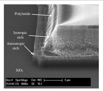
Figure 2.19: Polyimide edge profile after two-step plasma etching.
