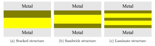
Figure 3.2: Approaches to dielectric layer stacking.
