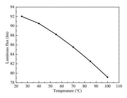
Figure 5.14: Luminous flux of the device as a function of temperature.
