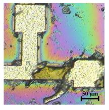
Figure 2.18: Interconnect delamination from PI.
