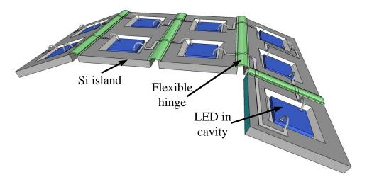
Figure 1.11: Silicon based flexible WLP package concept.
