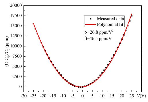
Figure 3.1: C-V characteristic of MIM capacitor with 95 nm Al<sub>2</sub>O<sub>3</sub> dielectric layer. The VCC parameters are extracted by fitting eq. (3.2).
