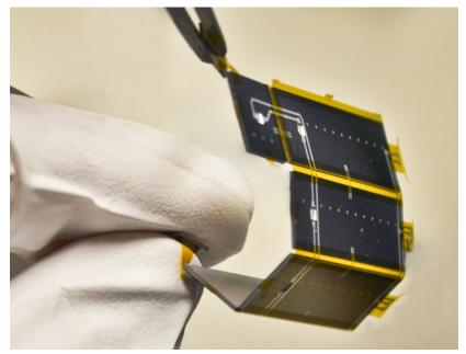
Figure 4.7: Flexible package released from wafer.
