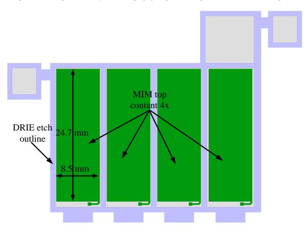
Figure 3.5: Backside layout of proposed WLP design, showing the dimensions of MIM capacitors.
