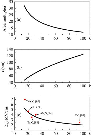
Figure 3.16: Design space requirements to integrate a 68  $\mu$ F, 25 V 3D capacitor in terms of (a) effective area, (b) layer thickness, (c) breakdown strength. Experimental results reported in [92, 93, 94] are added to (c) indicating the validity of the  $E_{bd} \sim k^{(-1/2)}$  model.
