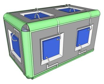
Figure 1.12: Flexible WLP design folded to form a cuboid.
