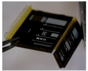
Figure 2.24: Flexible test chip.
