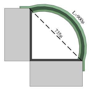
Figure 2.10: Schematic representation of right angle bend with arc-shaped polyimide hinge.
