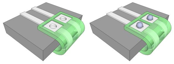
(a) Backside view of bondpads with cavities (b) Backside view with solder balls in cavities
