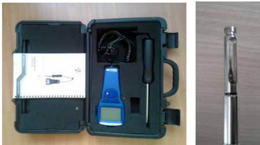
Figure 70: VelociCalc air velocity meter model 9515 (left) and the hot wire air velocity sensor (right)
