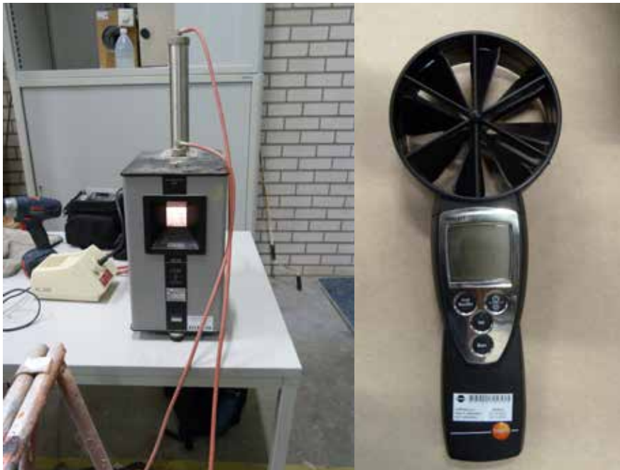
Figure 73: Betz 2500 micro manometer (left) and the Testo 417 vane anemometer (right)
