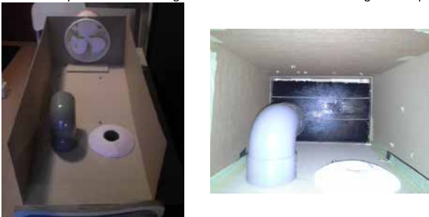
Figure 68: Wind tunnel setup with the fan (left) and the diffuser (right) visible.
