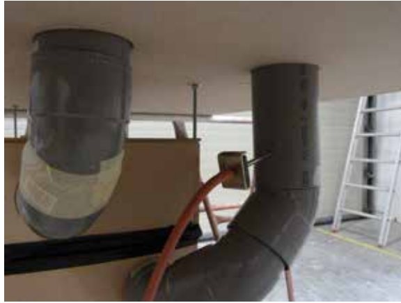
Figure 74: Pitot tube inserted into the pipes.
