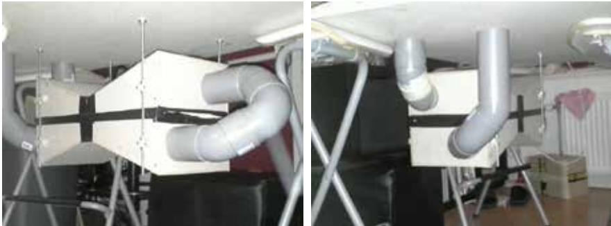
Figure 67: Heat exchanger mock-up. Scale 1:1.
