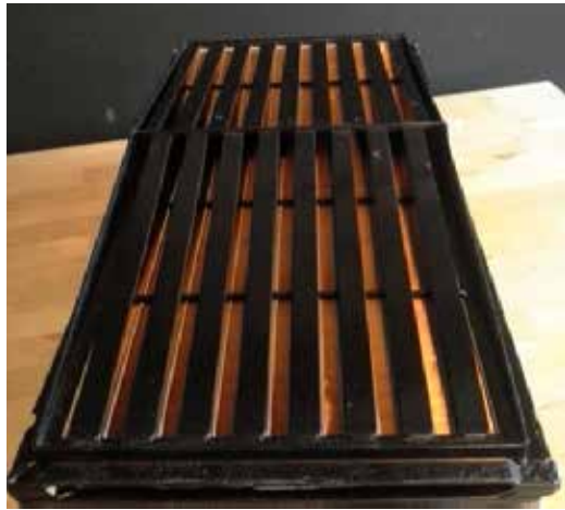
Figure 24: Fiwihex system air to air heat transfer.
