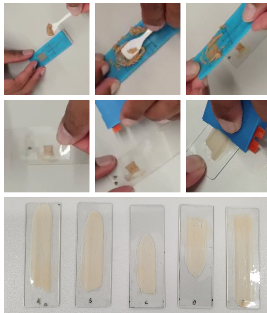
Figure 18: Steps showing the filtration and smearing processes using the prototype. As can be seen, fecal deposits were inconsistent due to flexibility of silicone
