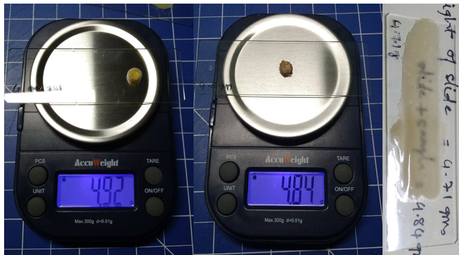
Figure 16: The weights of filtered fecal deposits consistently measure 40mg, showing that the sythetic feces created is reliable for testing
