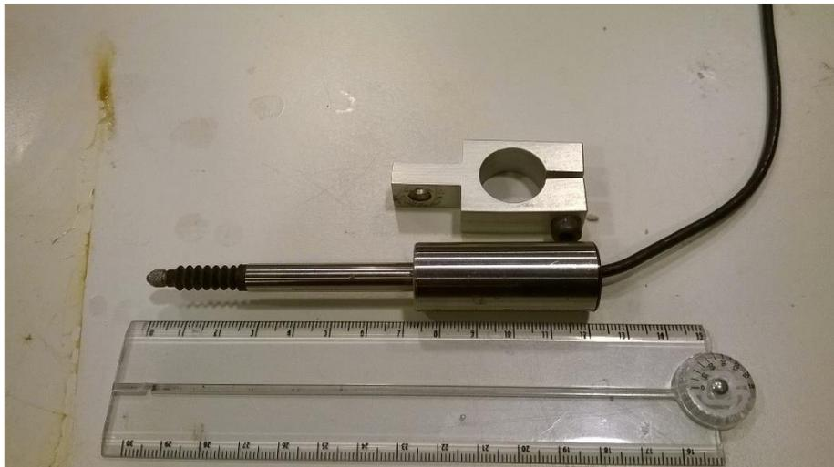
Figure 3-9 LVDT and Clamp System
