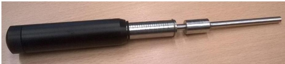
Figure 3-12 Modified Pocket Penetrometer
