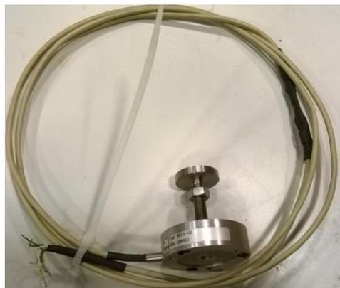
Figure 3-8 Load Cell Used in the Model
