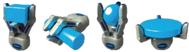
Fig. 6. Schunk SDH performing a range of distinct grasp types, adapted from [17]. In order from left to right are shown: parallel-, cylinder-, sphere-, and disk grasp.
