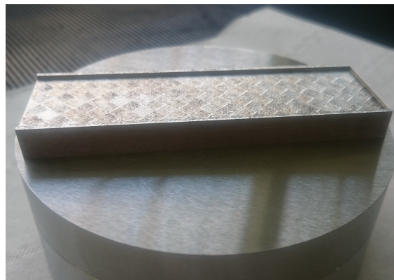
Figure 3.12: Positioning mould for 3D printing
