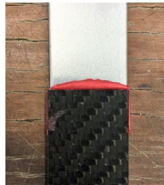
Figure 3.5: Adhesive reference joint with Aluminum and CFRP-1
