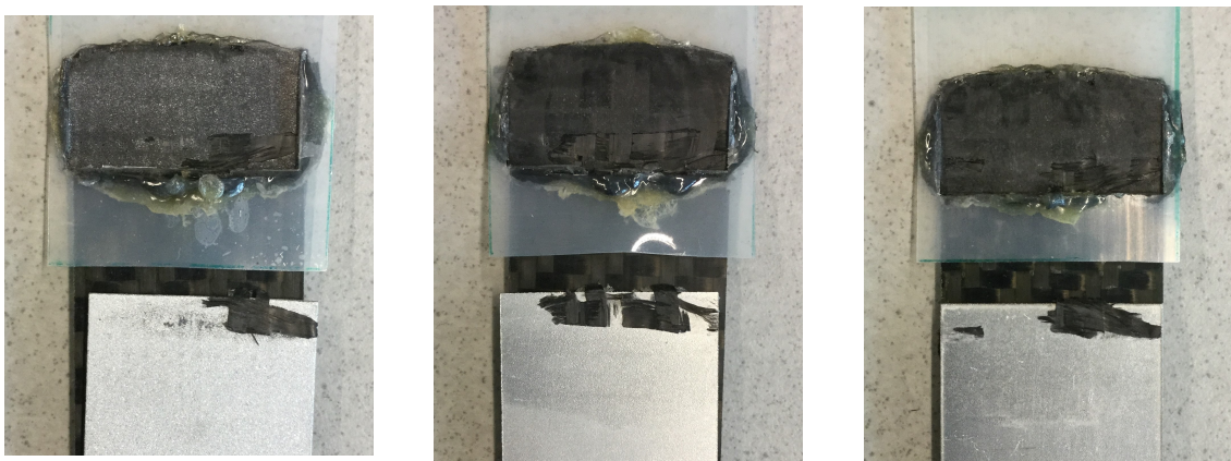
Figure 5.15: Fracture surfaces of joints between CFRP_1 and aluminum treated with sandblasting (left), conversion coating (center) and plasma (right). Larger area covered by fibers is present on the aluminum overlap compared to untreated samples
