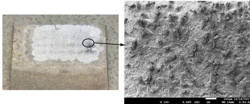
Figure 6.4: Fracture surface of sandblasted aluminum after artificial aging, inspected both visually and with SEM
