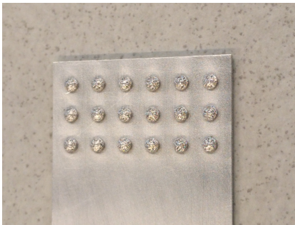
Figure 3.13: 3D printed pins on Al sample
