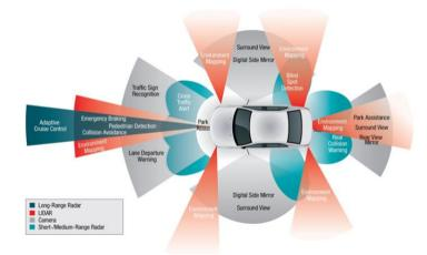
Figure 3.7: The cameras and sensors of an autonomous car (Wendt and Cook, 2018)
