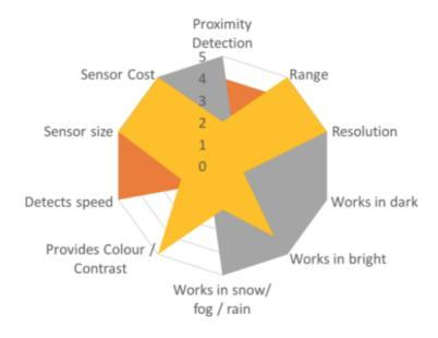
Figure 5.1: The abilities and disabilities of all sensors — LiDAR, short-range and long-range radar, cameras — combined (Barnard, 2016)
