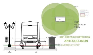
Figure 3.11. The static dimensions of the Easymile (Boersma, Van Arem, Rieck, 2018)
