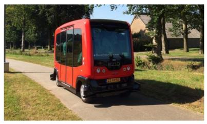
Figure 6.3: The Easymile EZ10 shuttle used in the Appelscha project (Boersma, van Arem, and Rieck, 2018)
