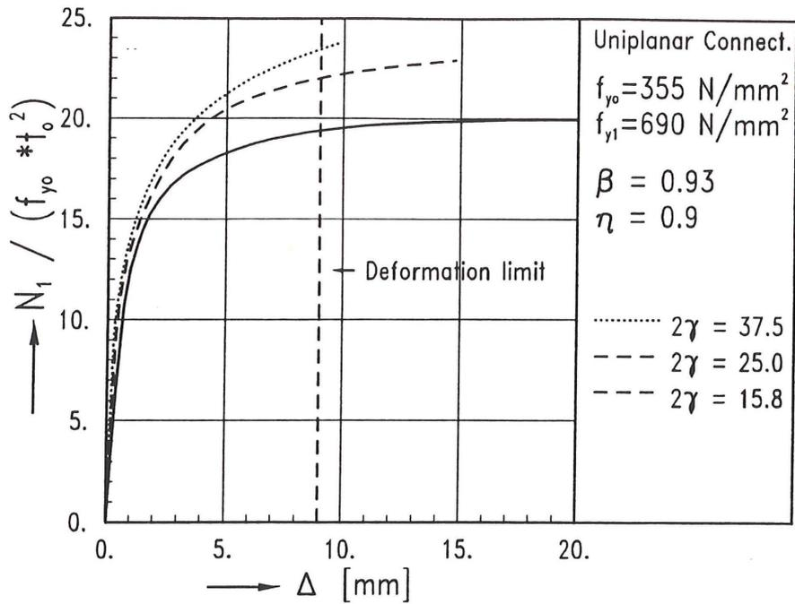
Fig. 6 Load - displacement curves for xb10a-xb12a
