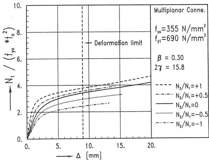
Fig. 11 Load - displacement curves for xxp1
