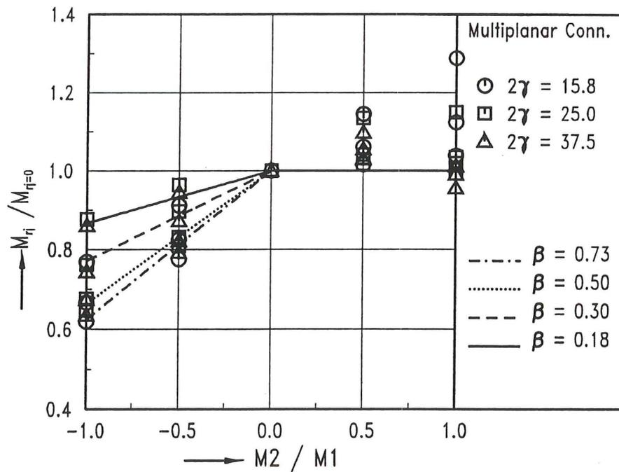
Fig. 31 Multiplanar load interaction effects
