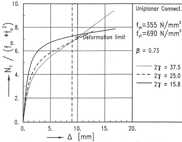
Fig. 6 Load - displacement curves for  $\beta = 0.73$
