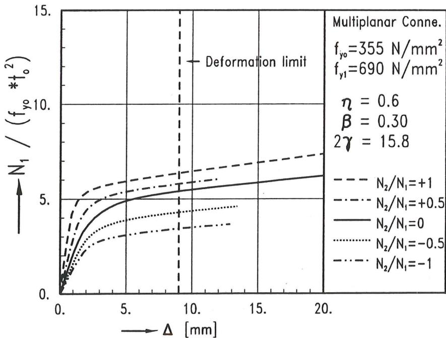
Fig. 9 Load - displacement curves for xxb1a
