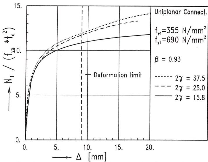
Fig. 7 Load - displacement curves for  $\beta = 0.93$
