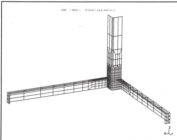
Figure 1 Typical finite element mesh for a multiplanar connection (xxb5a)
