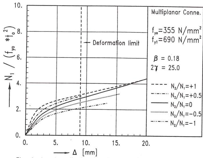
Fig. 9 Load - displacement curves for xxp14
