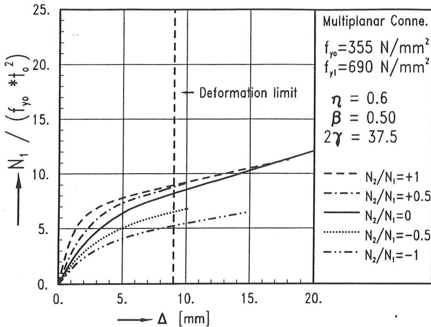
Fig. 14 Load - displacement curves for xxb6a
