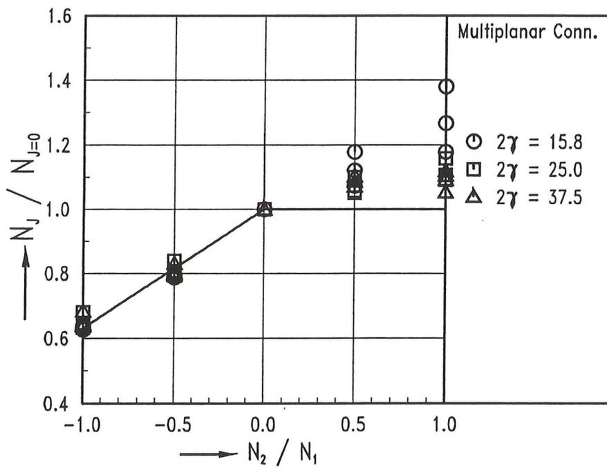
Fig. 6 Multiplanar load interaction effect
