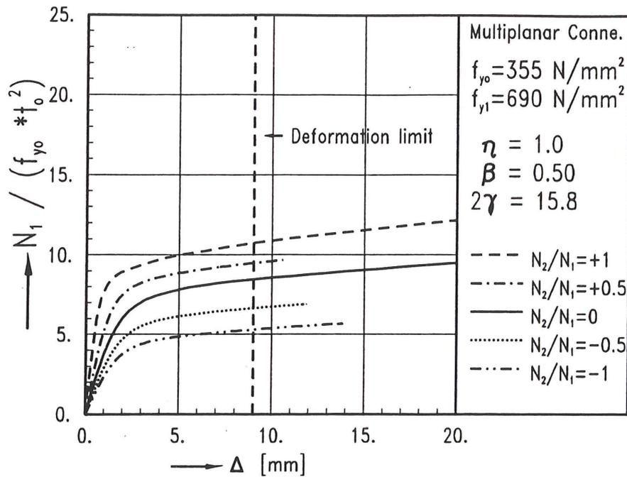
Fig. 12 Load - displacement curves for xxb4a
