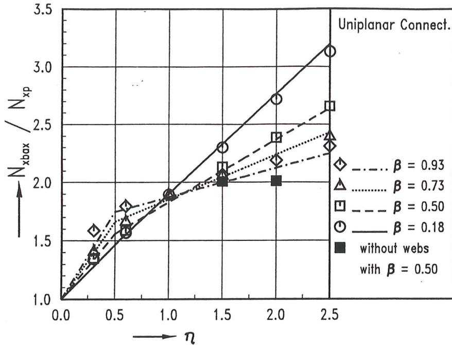
Fig. 4 The effect of the second flange and web
