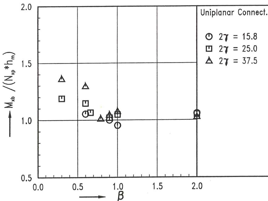
Fig. 29 Comparisons between I-beam to RHS column and corresponding plate to RHS connections
