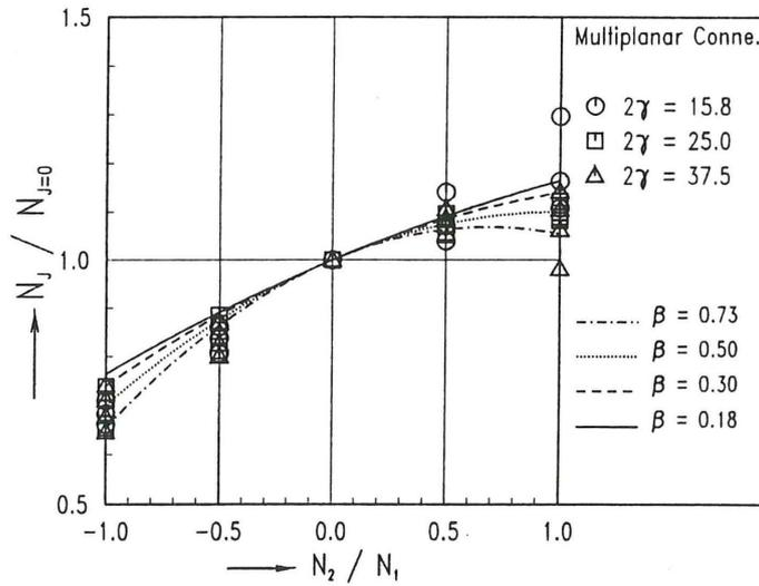
Fig. 22 Multiplanar load interaction effects
