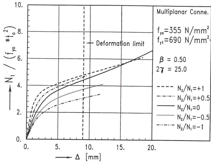
Fig. 15 Load - displacement curves for xxp5
