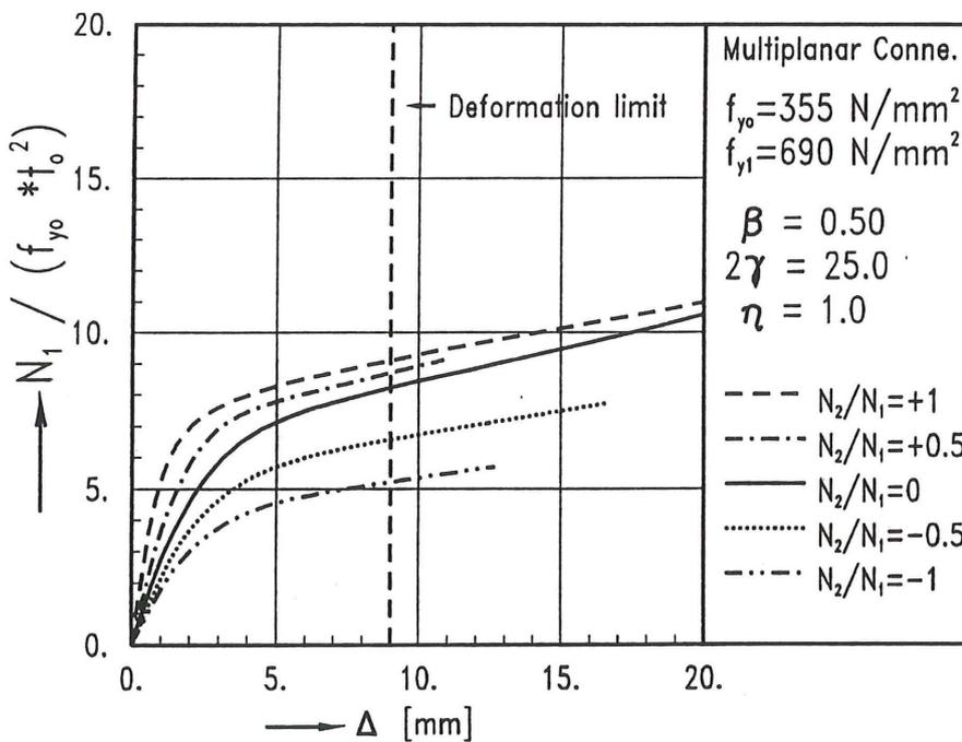
Fig. 3 Load - displacement curves for xxb5a
