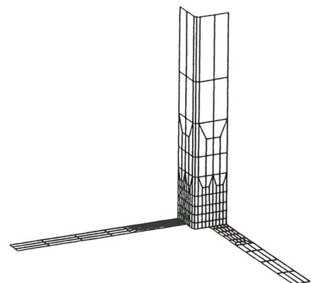
Figure 2 Typical Finite element meshes for a multiplanar connection xxp5
