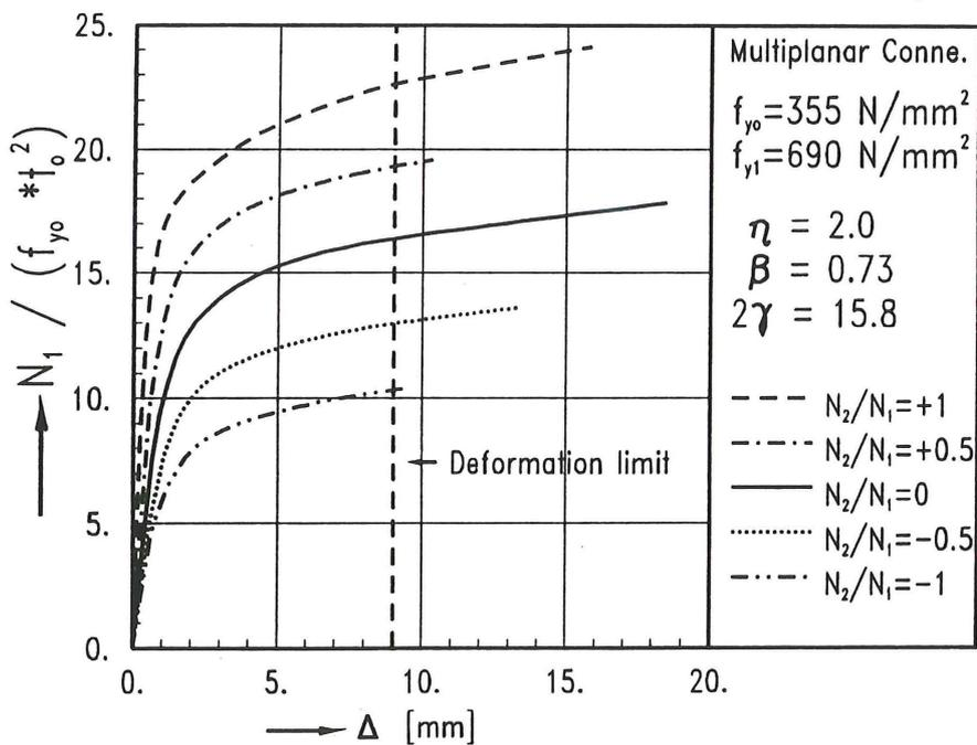
Fig. 15 Load - displacement curves for xxb7a
