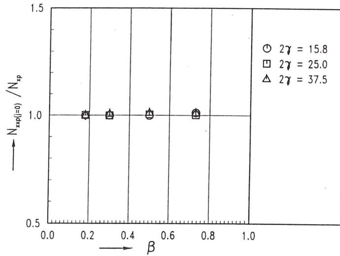
Fig. 21 Comparisons between multiplanar connections with  $J=0$  and corresponding uniplanar connections
