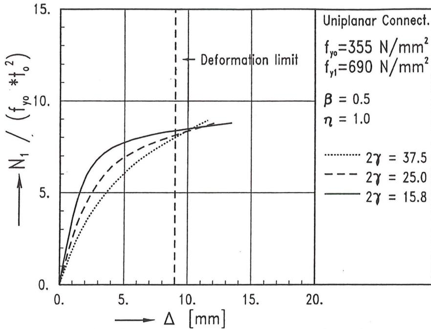
Fig. 2 Load - displacement curves for  $\beta = 0.50$
