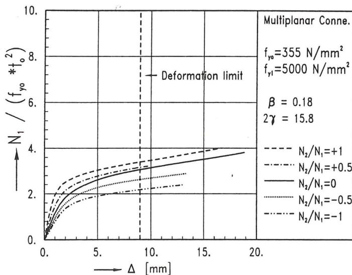
Fig. 8 Load - displacement curves for xxp13
