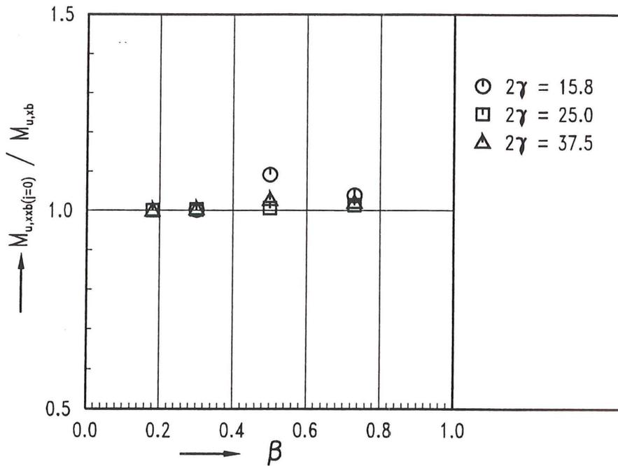
Fig. 30 Comparisons between multiplanar connections with  $J=0$  and corresponding uniplanar connections
