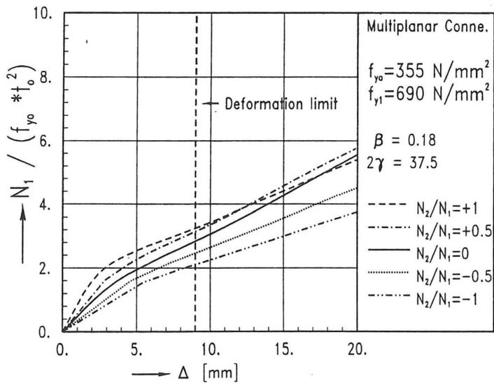
Fig. 10 Load - displacement curves for xxp15
