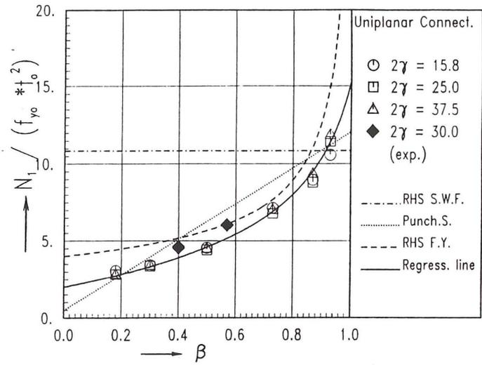
Fig. 20 The influence of  $\beta$  on the strength of uniplanar plate to RHS connections
