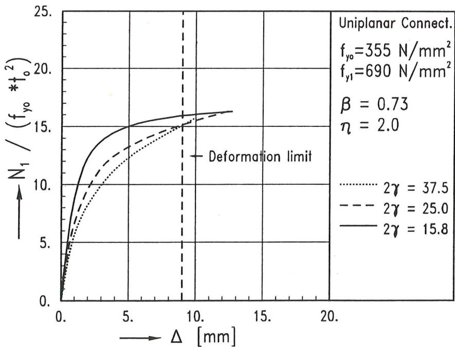
Fig. 5 Load - displacement curves for xb7a-xb9a
