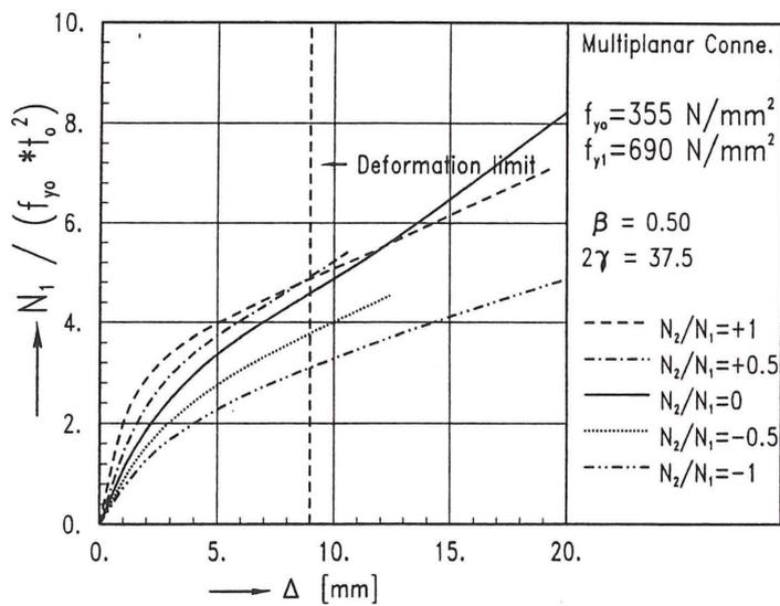
Fig. 16 Load - displacement curves for xxp6
