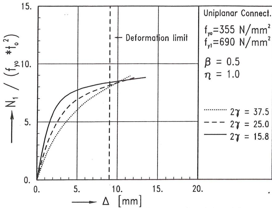
Fig. 4 Load - displacement curves for xb4a-xb6a
