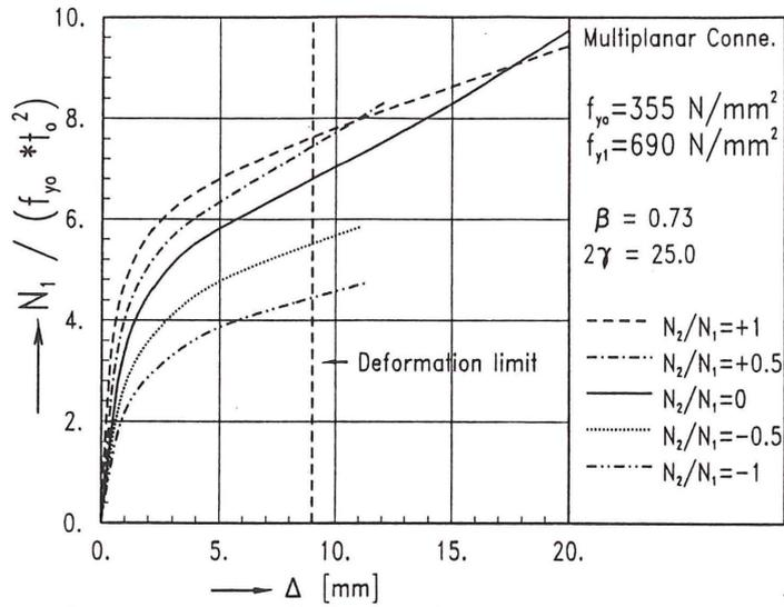
Fig. 18 Load - displacement curves for xyp8
