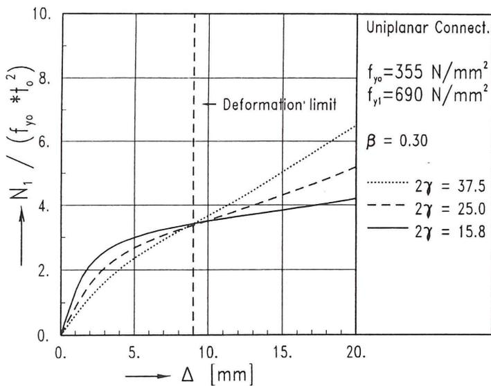
Fig. 4 Load - displacement curves for  $\beta = 0.3$
