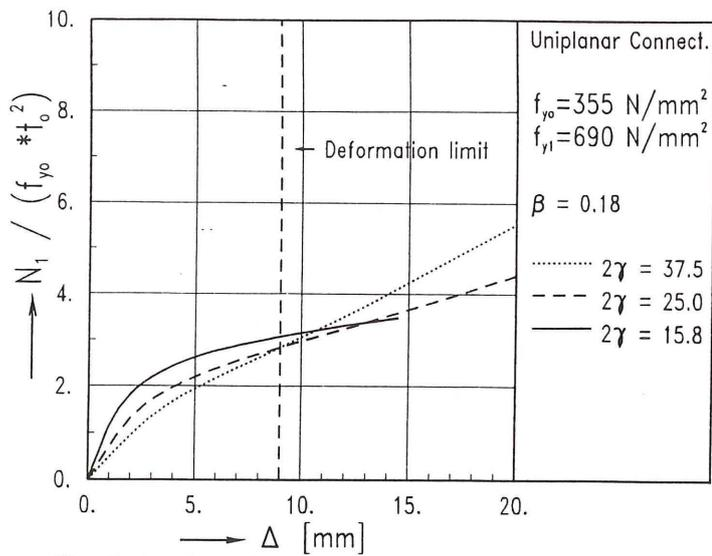
Fig. 3 Load - displacement curves for  $\beta = 0.18$
