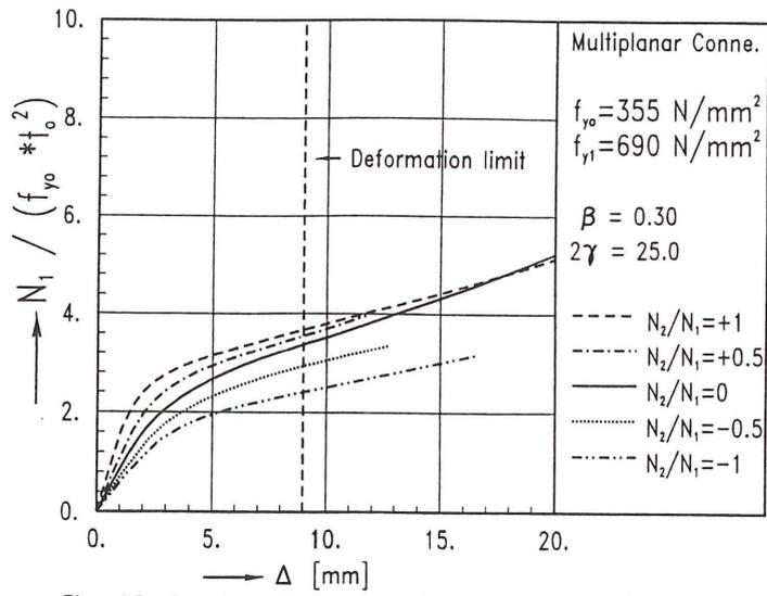
Fig. 12 Load - displacement curves for xxp2
