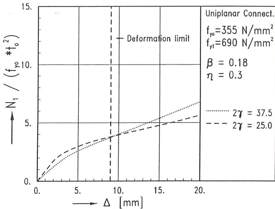
Fig. 2 Load - displacement curves for xb14a-xb15a
