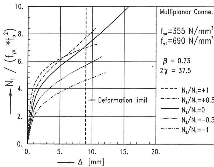
Fig. 19 Load - displacement curves for xyp9
