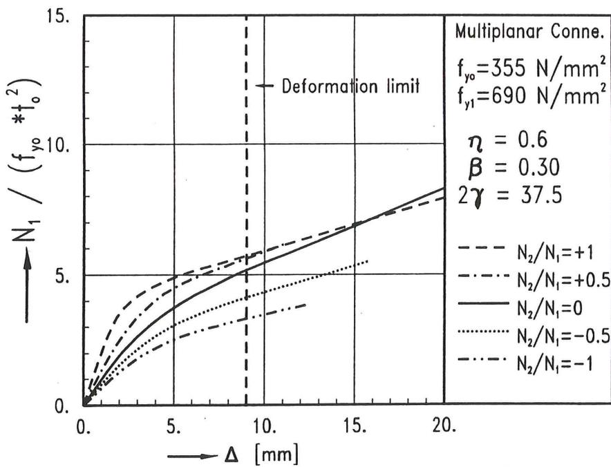
Fig. 11 Load - displacement curves for xxb3a
