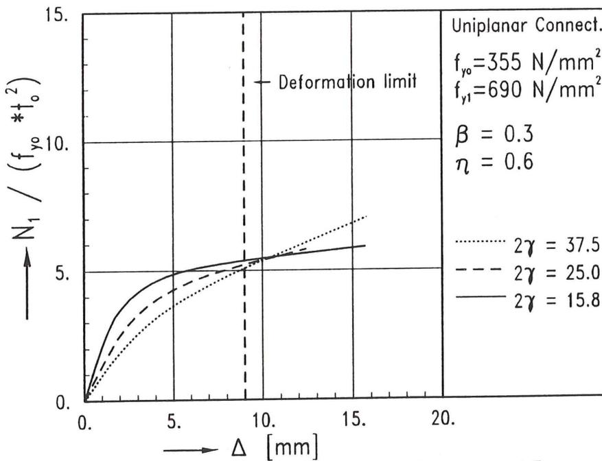
Fig. 3 Load - displacement curves for xb1a-xb3a
