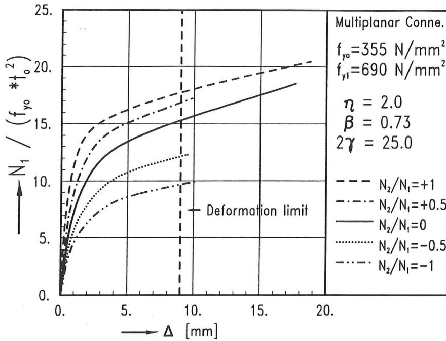
Fig. 16 Load - displacement curves for xxb8a
