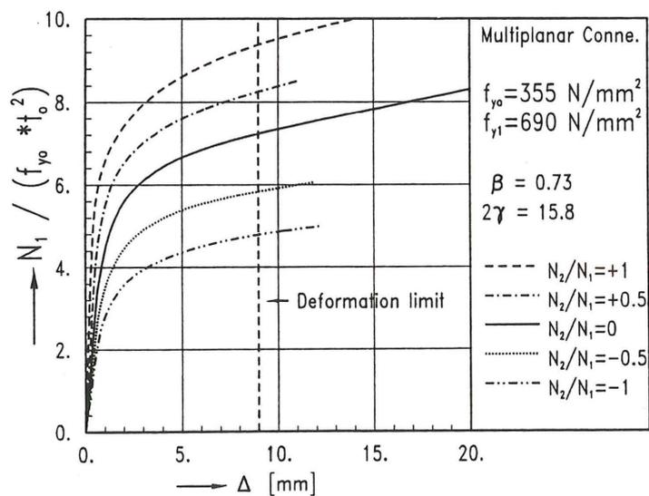
Fig. 17 Load - displacement curves for xxp7
