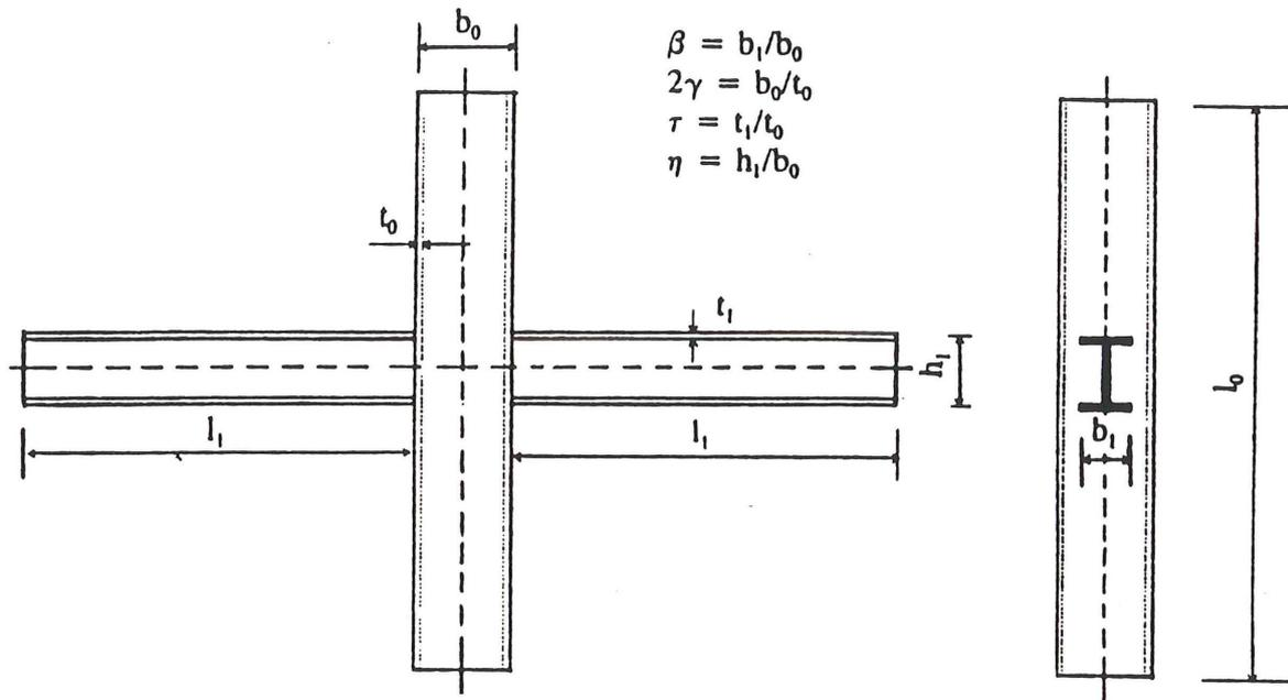
Fig. 1 Configuration of plate or I-beam to RHS column connection
