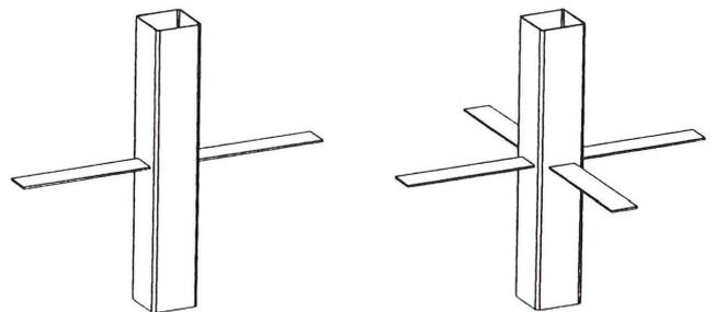
Figure 1 Configurations of plate to RHS column connections
