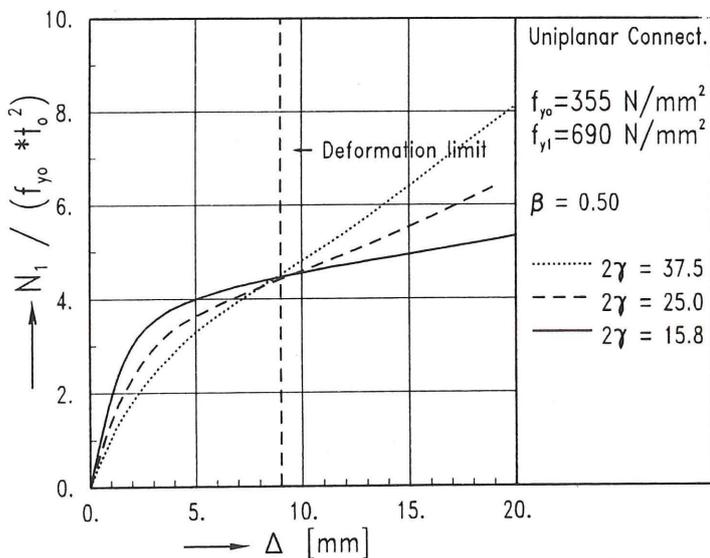
Fig. 5 Load - displacement curves for  $\beta = 0.5$
