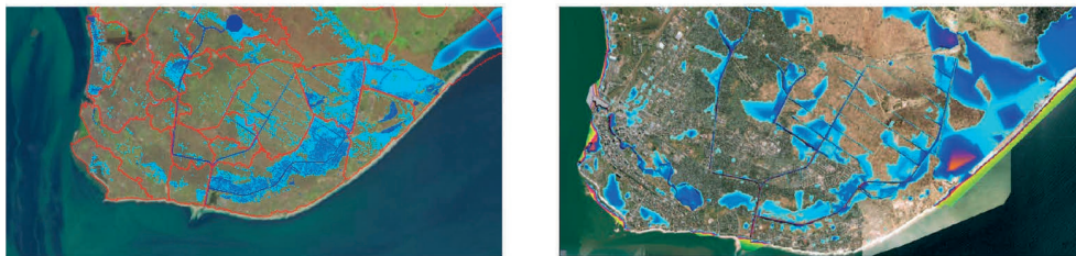
Figure 3-5: flood extent resulting from a 10 year rainfall event for FLORES (left) and an ANUGA simulation, which was part of the Rio Chiveve feasibility study. Background image: Sentinel-2 (© ESA).
