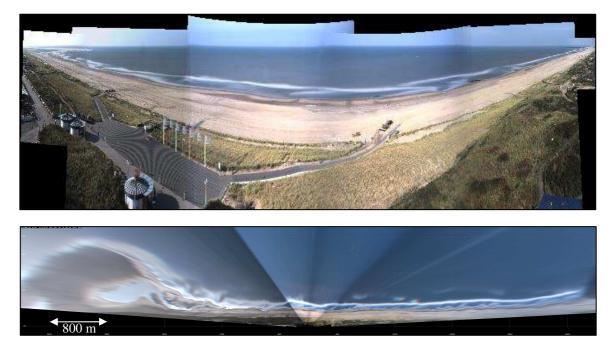
Figure 2: Merged (upper) and rectified (lower) time exposure image capturing leeside of Sand Engine from Kijkduin.
