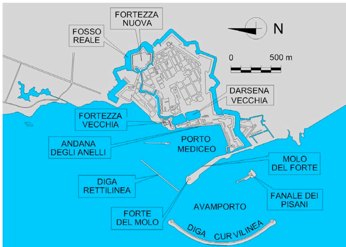
Figure 6. Project of the Diga Curvilinea (Curvilinear Breakwater) and of the Diga Rettilinea (Straight Breakwater) of the Poirel (1851).
