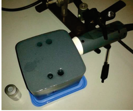
FIGURE 1. Photograph of the setup with a block of tissue mimicking material with cavities, and the probe imaging the region.
