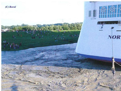
Fig. 21: Evolution of estuarine turbidity maximum in Ems River (upper panel; after de Jonge, 2009) with suspended sediment concentrations up to 40 g/l. The left panel depicts conditions in the river upon passage of a cruise ship, built at the wharf at Papenburg, near the head of the river.
