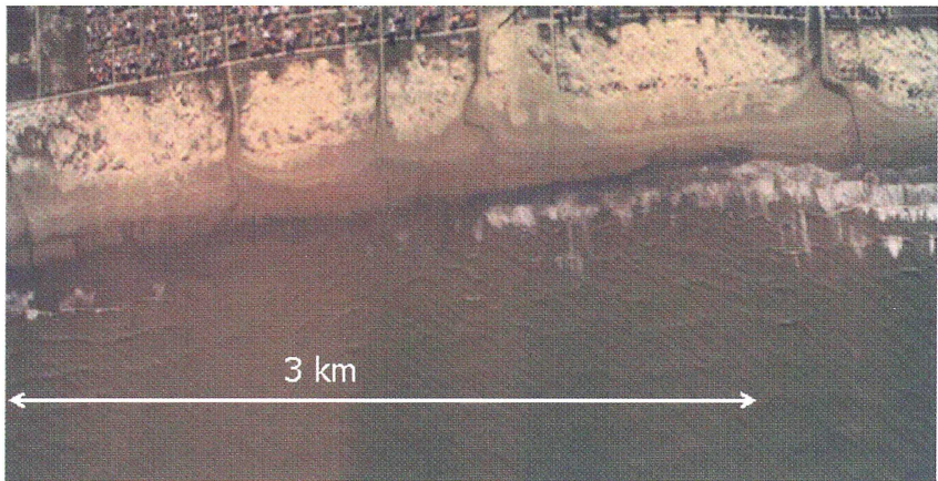
Fig. 5: Fluid mud induced wave damping (note foam generated by breaking waves in right-hand side of the photograph) at Cassino Beach, Brazil. The left panel shows landing of mobile fluid mud on the beach.
