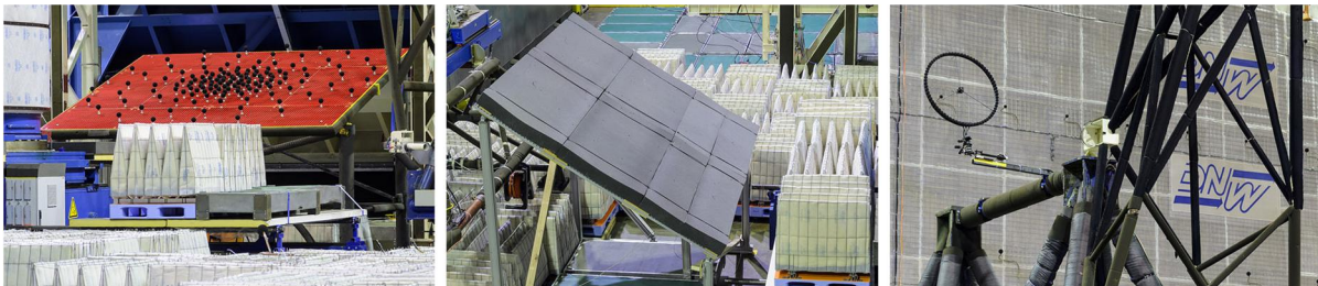
Figure 8: Microphone arrays from DNW (left), DUT (center), and INCAS (right).
