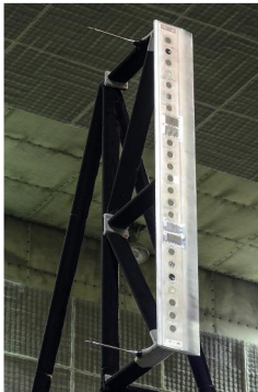
Figure 6: Traversable inflow acoustic instrumentation.
