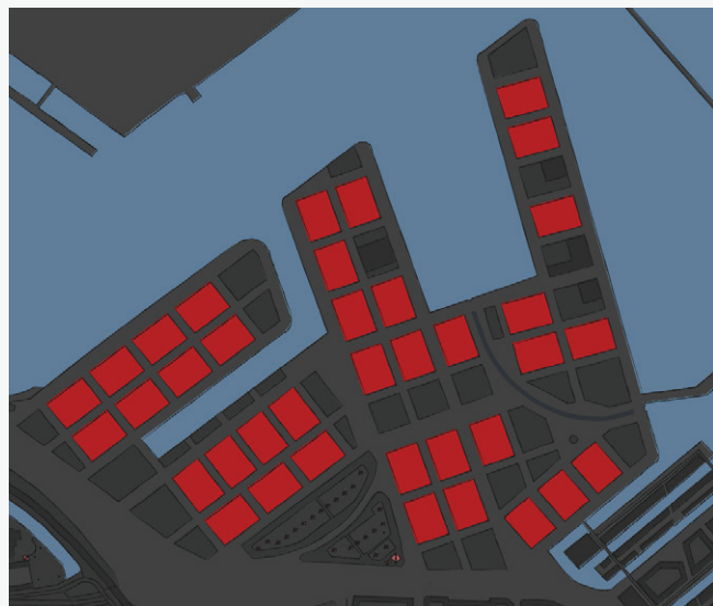
Image 5.1.2: Blocks with the standard sizes in the new design for the Minerva city-harbour.
