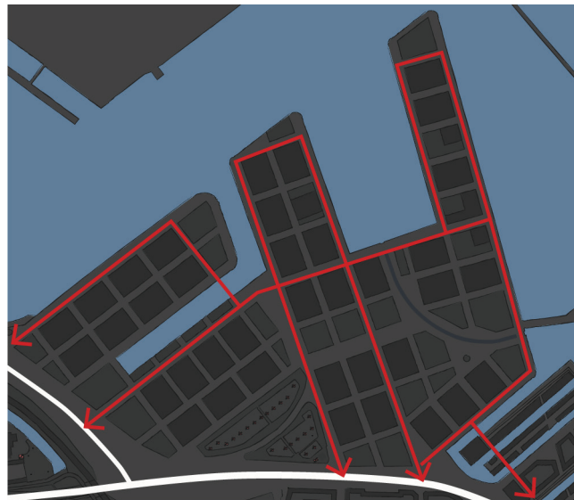
Image 5.1.8: Main access structure for cars in the new design for the Minerva city-harbour.
