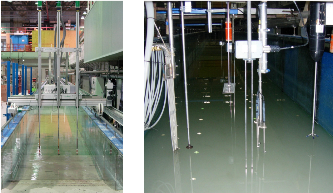
Figure 2. Left: bed profiler with three probes. Right: carriage with (from left to right): TSS, EMS, reference rod, WHM, ASTM and ADV.
