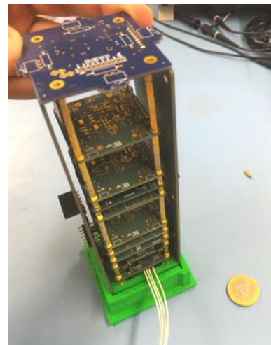
Figure 3. Stack approach for the inner structure of the final design
