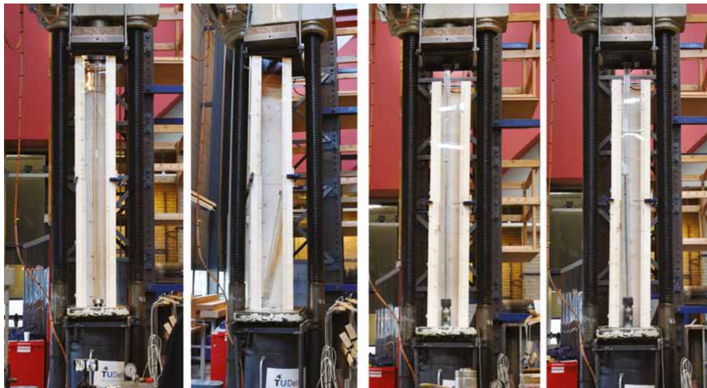
Fig.13: Left: A NT specimen prior and after failure. Right: A PT specimen prior and after failure.
