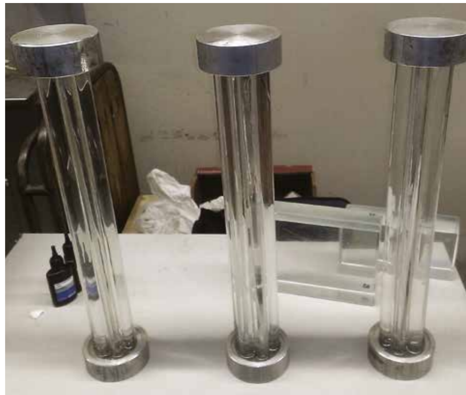
Fig.5: The 500 mm long specimen series tested in compression.
