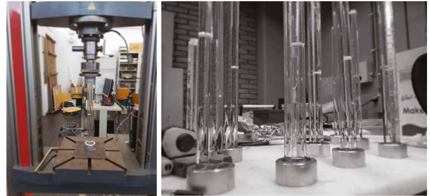
Fig.6: Left: Experimental set-up for the testing of alternative connections. Right: Specimens comprising two continuous rods and one interrupted in the middle.
