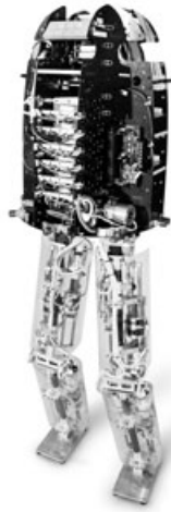
Figure 7.1: M2V2, a 3D force-controllable humanoid robot with twelve actuated degrees of freedom.
