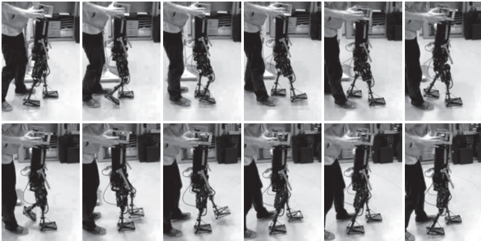
Figure 6.2: Images showing TULip performing a stride of a cyclic walking gait (Takahashi, 2009). The closeness of the operator gives away that small interventions are required every few steps to prevent a fall. Images are stills from the video visible on the Delft Biorobotics Laboratory website (Delft Biorobotics Laboratory, 2011).
