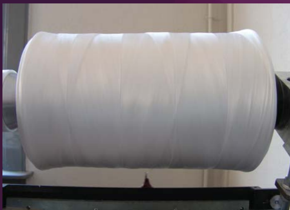
Figure 1: The 30 km of YES2 tether, a total of 5.5 kg only. The material is Dyneema, a Dutch invention and the same material that is used for kite-surfing.
