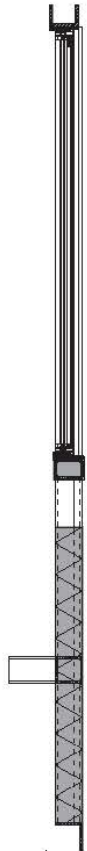
3-layer thermal glasses blinds between the glass panels ventilation vents in structure
