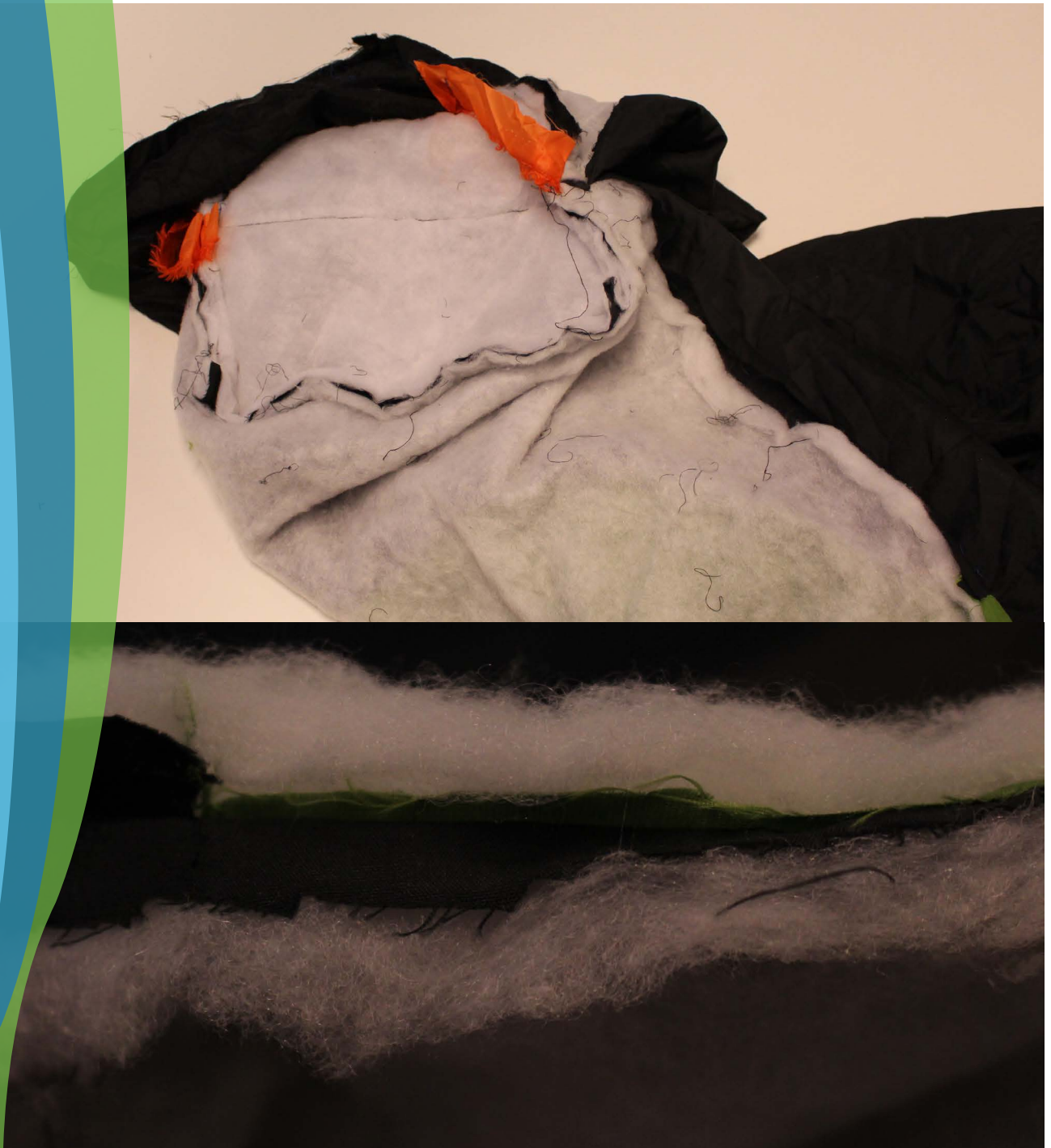
Figure 46 The connection between the lining and the outer fabric with insulation of the sleeping bag. This construction allows more freedom of movement for the user during the night.
