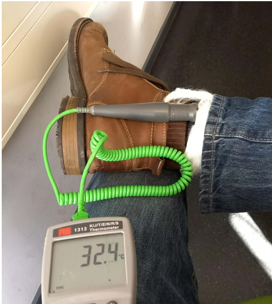
Figure 12 Measuring the temperature of the skin underneath the Dyneema fibre wrap, after walking up and down two staircases.
