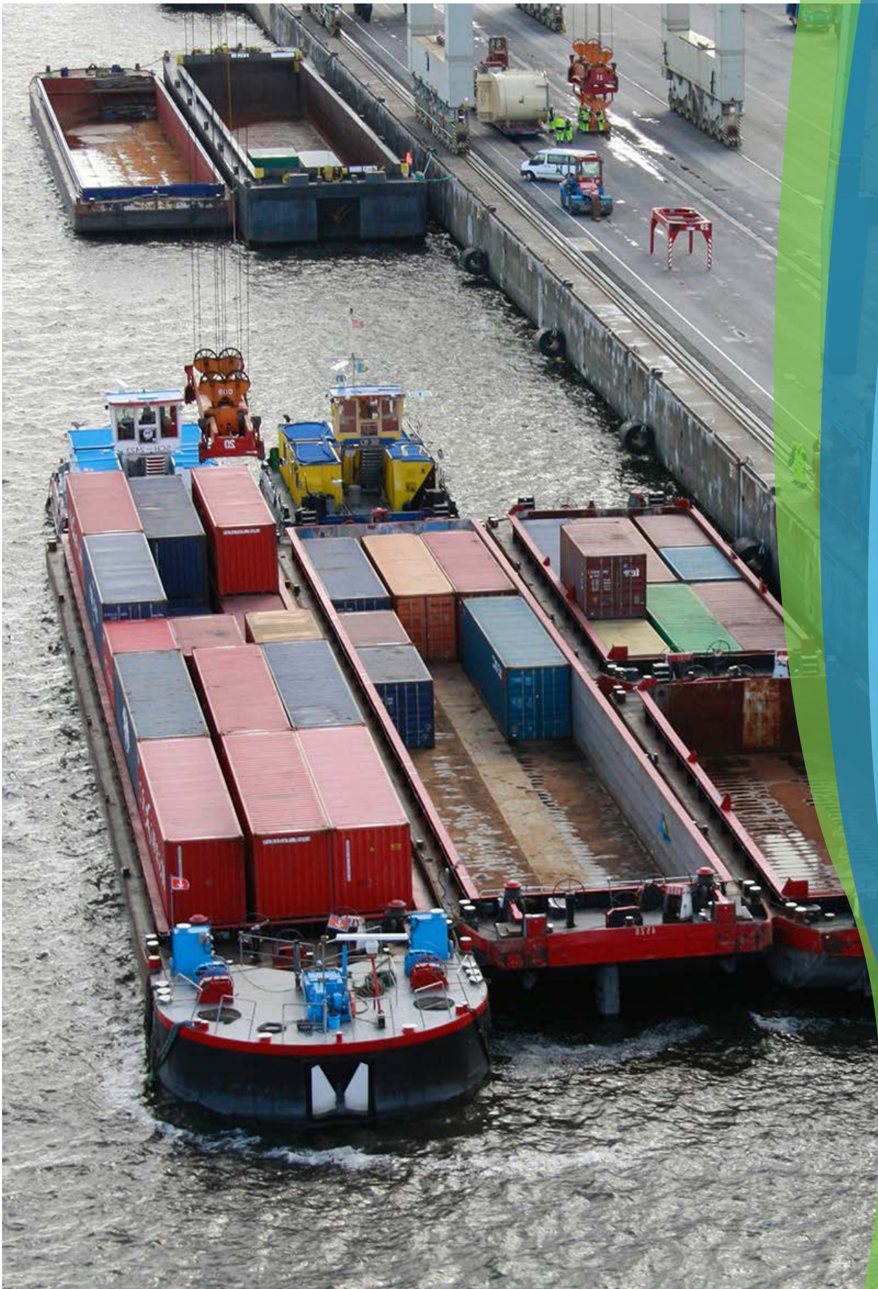
Figure 18 Container carrying inland ships, the containers lock onto each other. Therefore the need for ropes is far less than on multi-purpose dry cargo vessels.
