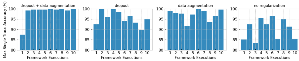
Figure 24: Random CNN hyperparameters: maximum single trace accuracy on the cswap-pointer dataset for ten different framework executions and attacking the sample interval range from 550 to 800 of all sub-traces.
