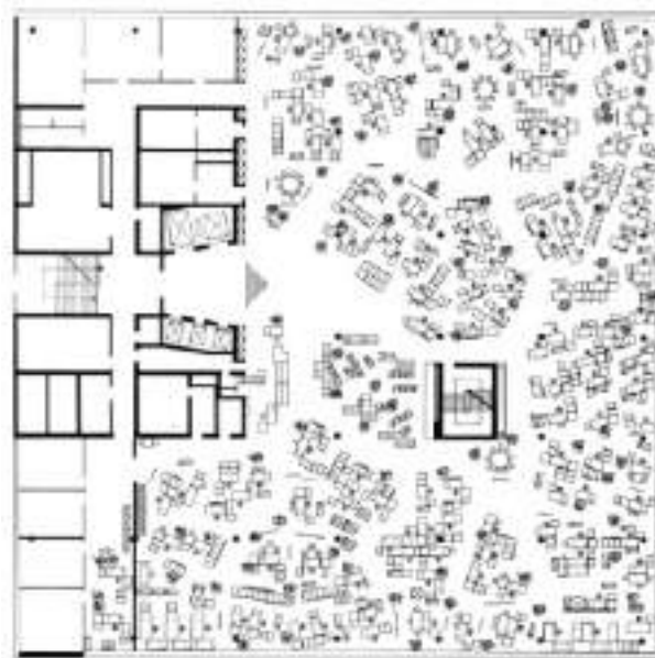
Fig. XX. Quickborner. (2022). Quickborner reintroduced the partition, but in an appropriately mobile, Semperian form, with their 'Bürolandschaft' [Illustration].
