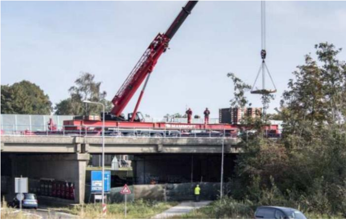
Figure 1: Pilot proof load test being performed on the Vechbrug in the Netherlands (October 2016).
